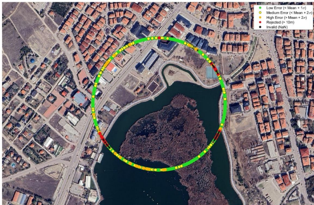
Figure 4.8. Results of the virtual position analysis for circular trajectory over satellite image
