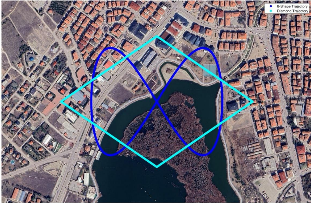
Figure 4.13. 8-shape and diamond trajectory of UAV used in the simulation over the satellite image
