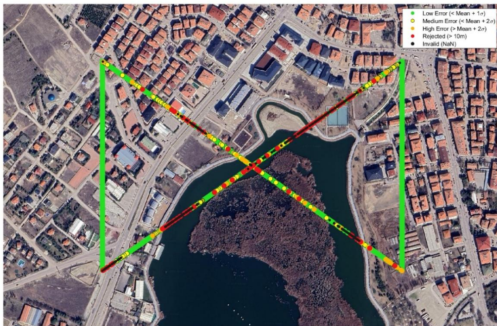
Figure 4.12. Results of the virtual position analysis for bowtie trajectory over satellite image
