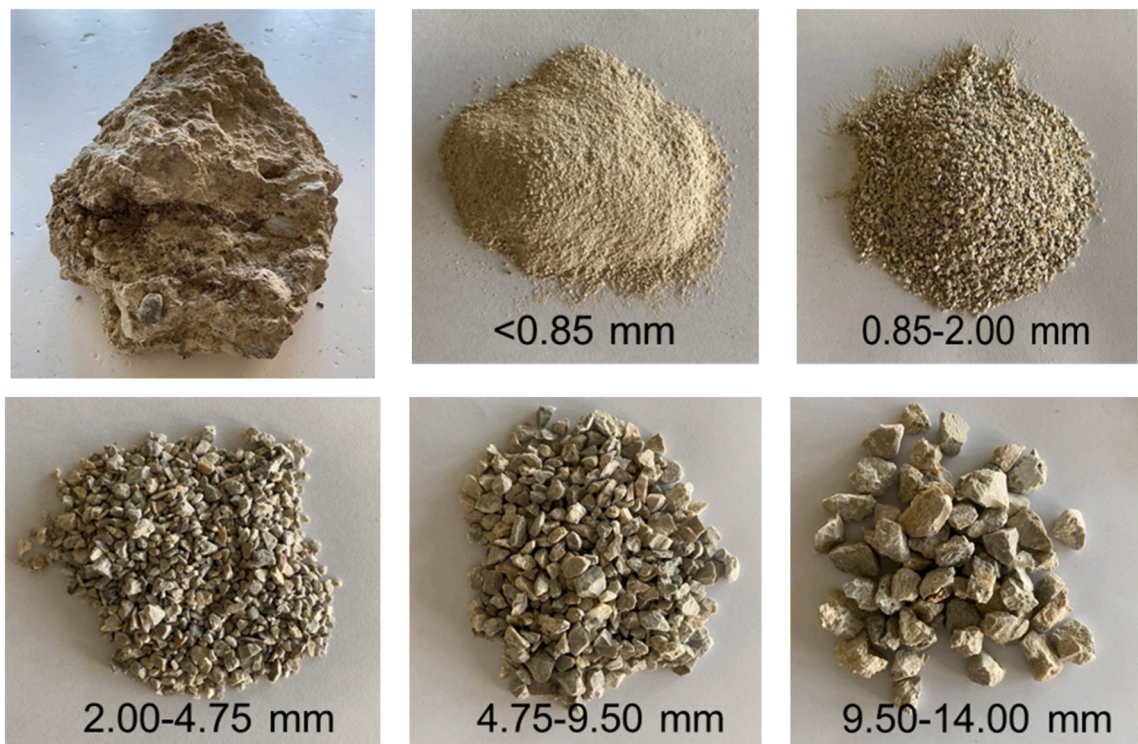
Fig. 1. Views of concrete rubbles and RCAs in different particle sizes.
