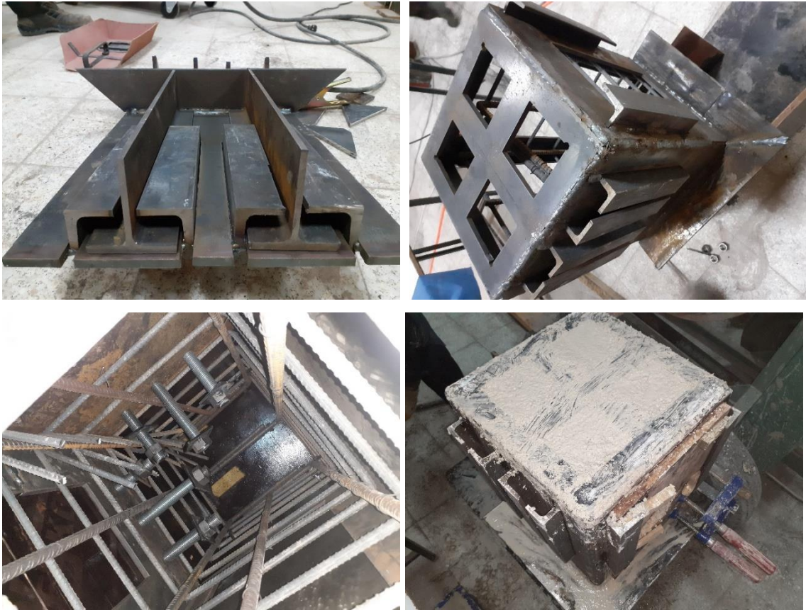
Figure 3.49 Details of demountable column head
