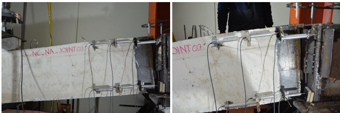
Figure 4.34 First cracks on the demountable beam connection
