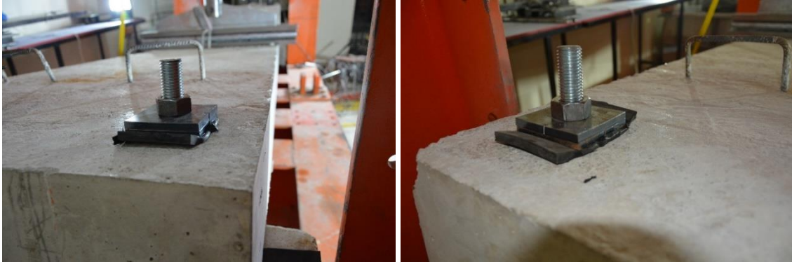
Figure 4.43 Elastomeric pads usage in the demountable slab-to-beam connection
