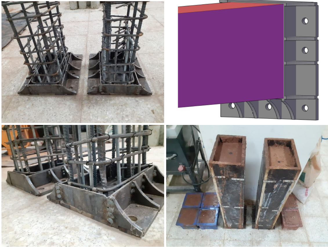
Figure 3.50 Details of primarily produced demountable beam specimen
