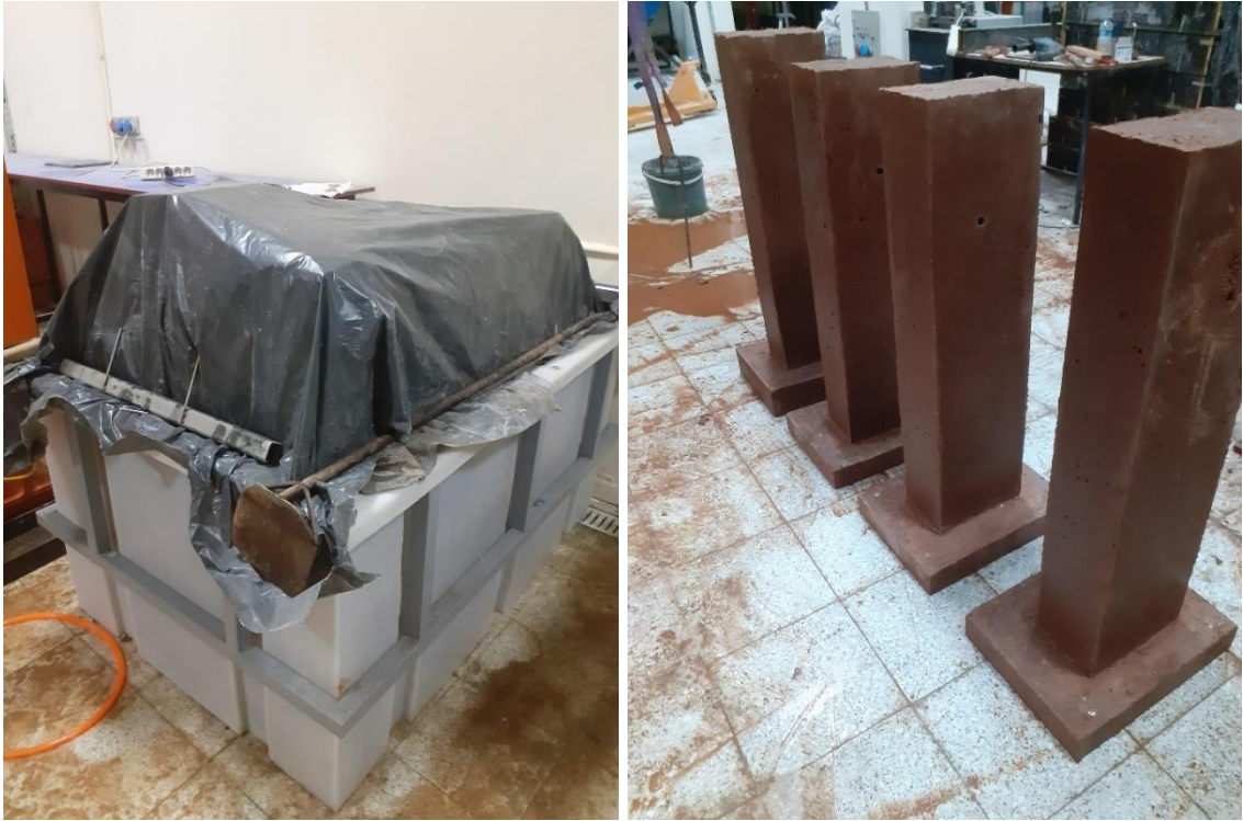
Figure 3.18 Curing of geopolymer demountable columns
