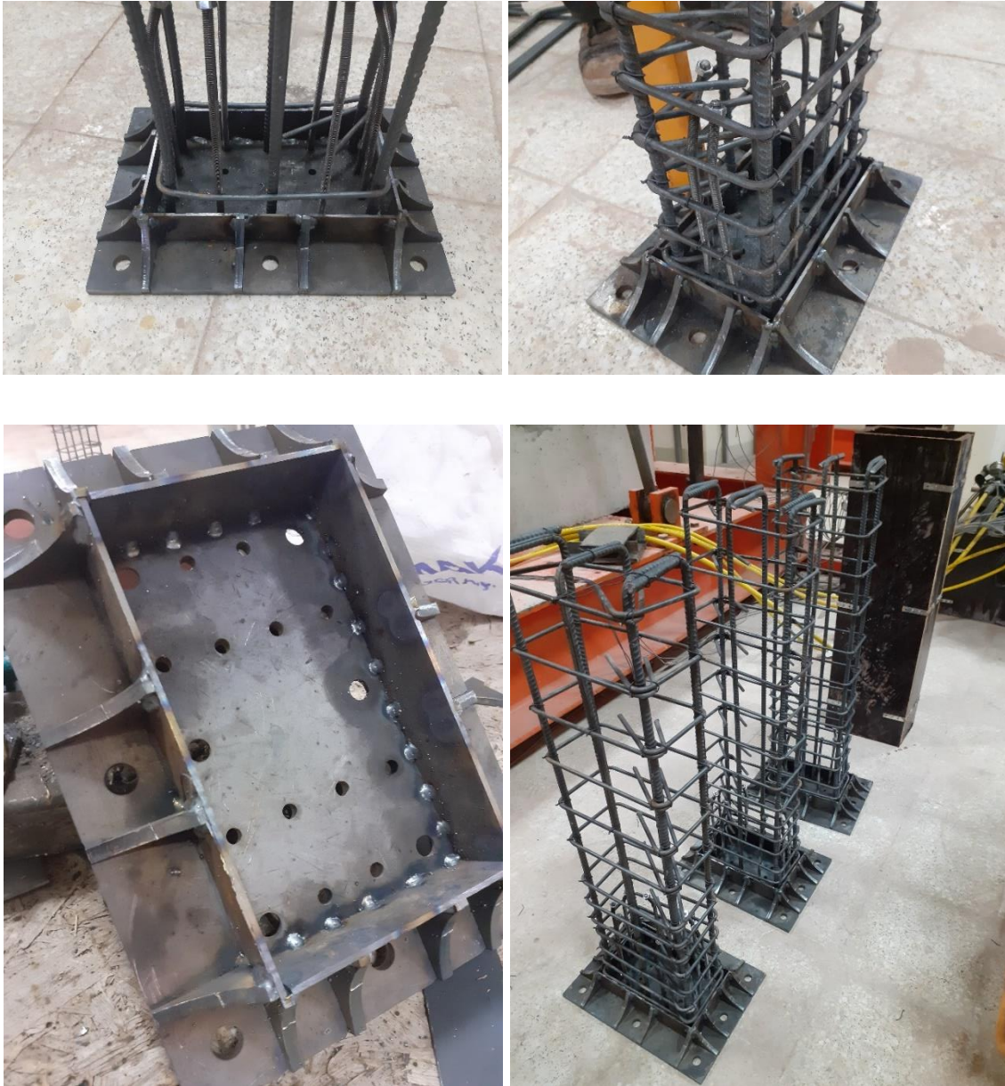
Figure 3.29 Details of demountable column 4 (DC4)
