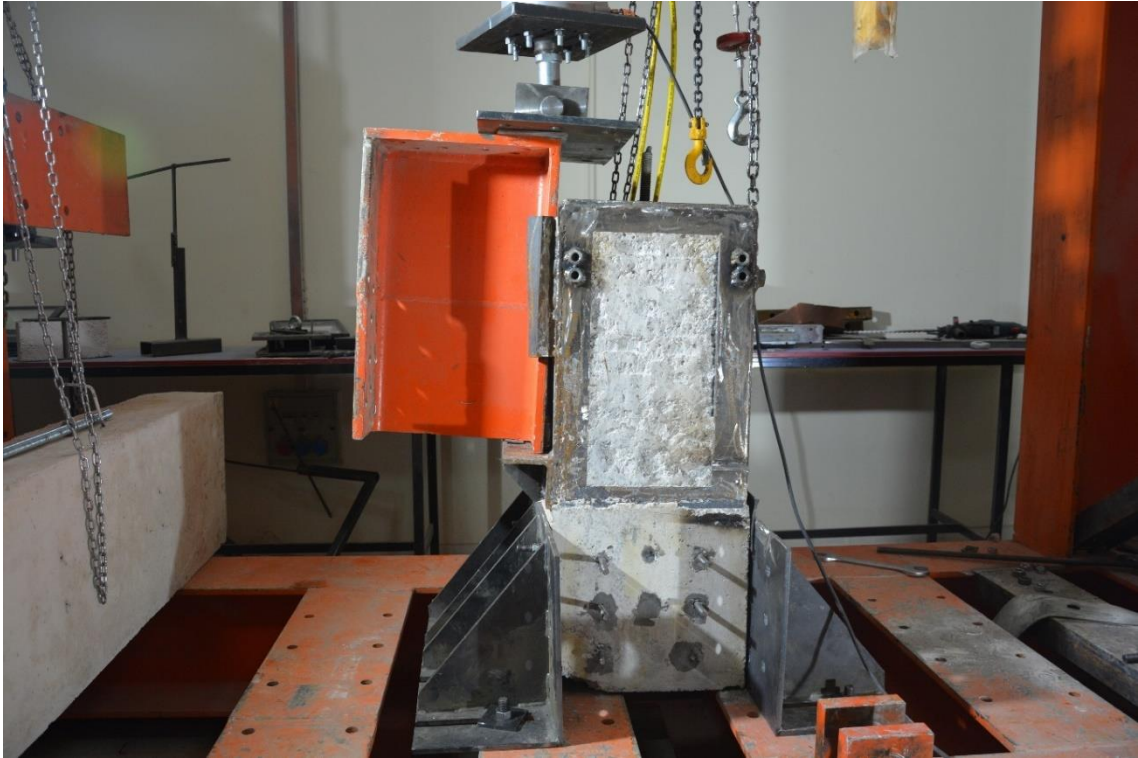
Figure 4.36 Shear test of the beam-to-column connection
