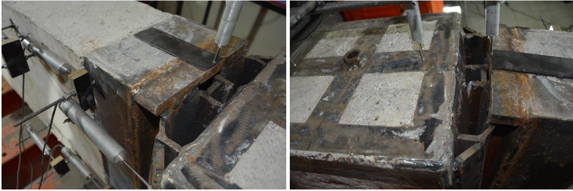
Figure 4.35 Failure states of the beam-to-column connection
