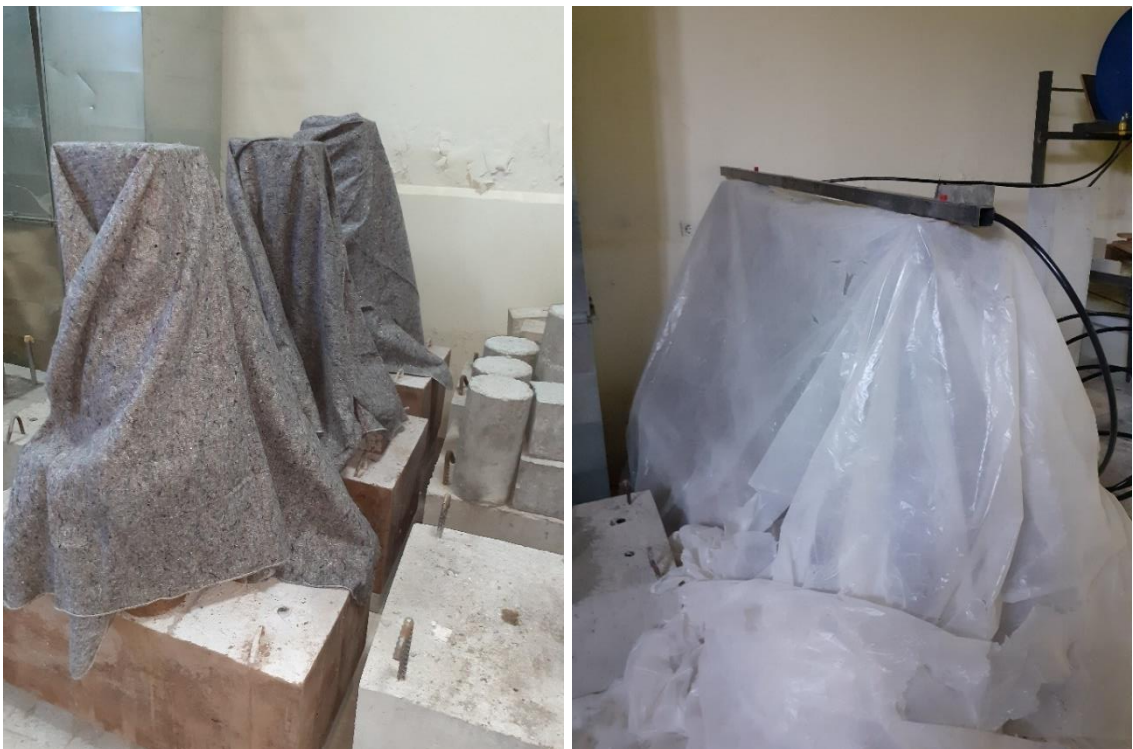
Figure 3.19 Curing of geopolymer monolithic columns with a drip system
