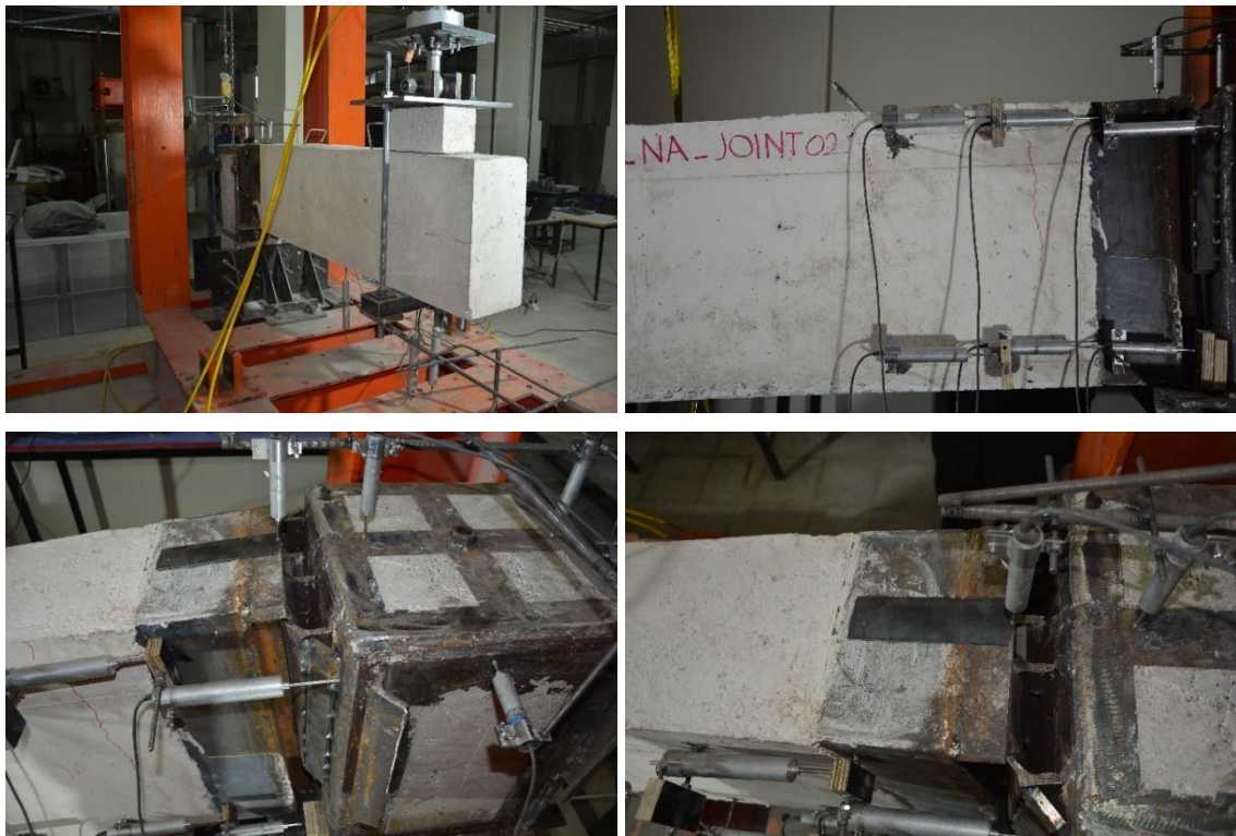
Figure 3.53 Flexural test setup of the demountable beam to column connection
