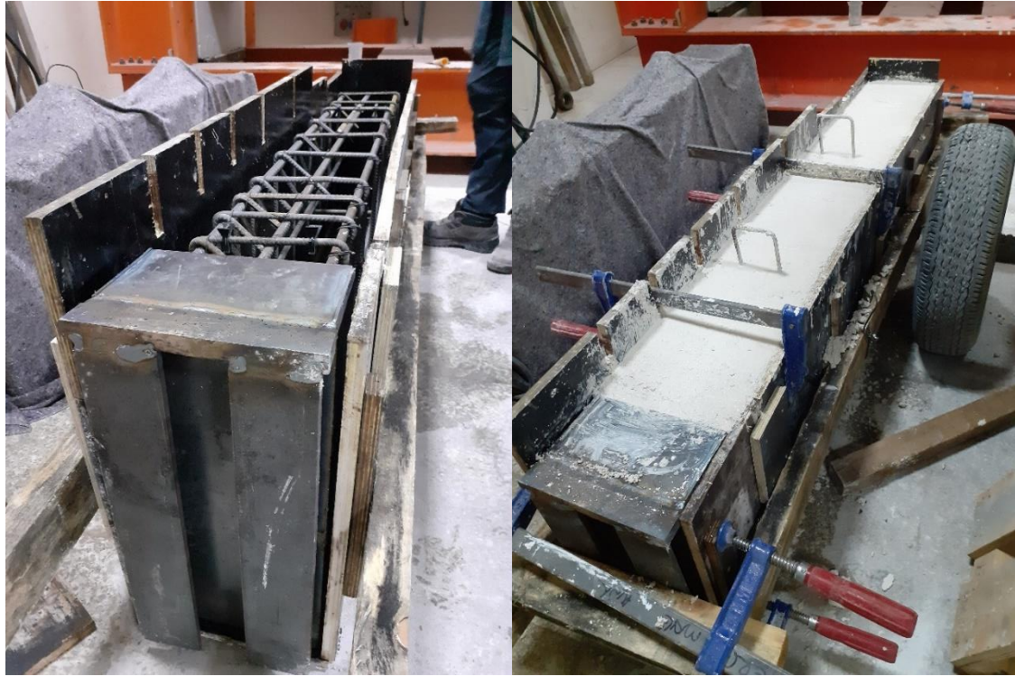
Figure 3.51 Preparation of pin-type demountable beams
