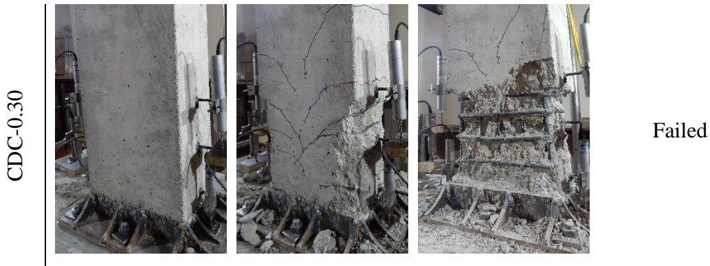
Figure 4.7 Damage progression in the bolted specimens with increasing drift ratio
