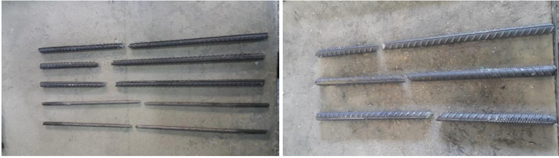
Figure 3.14 Tensile test of reinforcement bars
