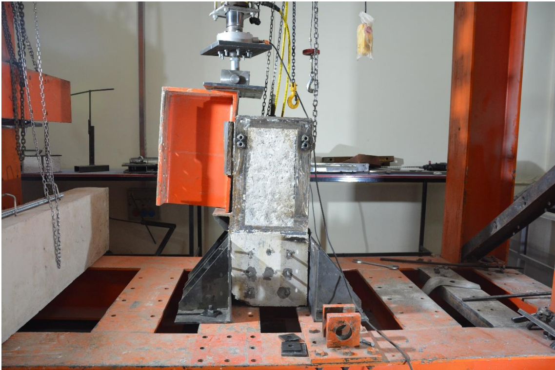
Figure 3.54 Shear test setup of the column head
