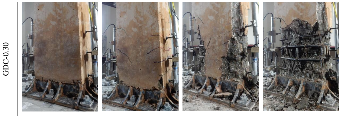
Figure 4.5 Observed failure modes at the demountable specimens.
