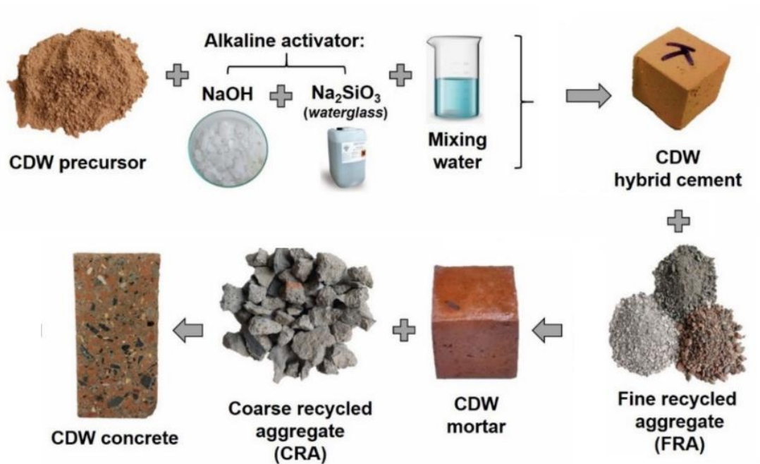
Figure 2.3 Steps involved in converting CDW precursors into CDW concrete (adapted from Robayo-Salazar et al. [56])
