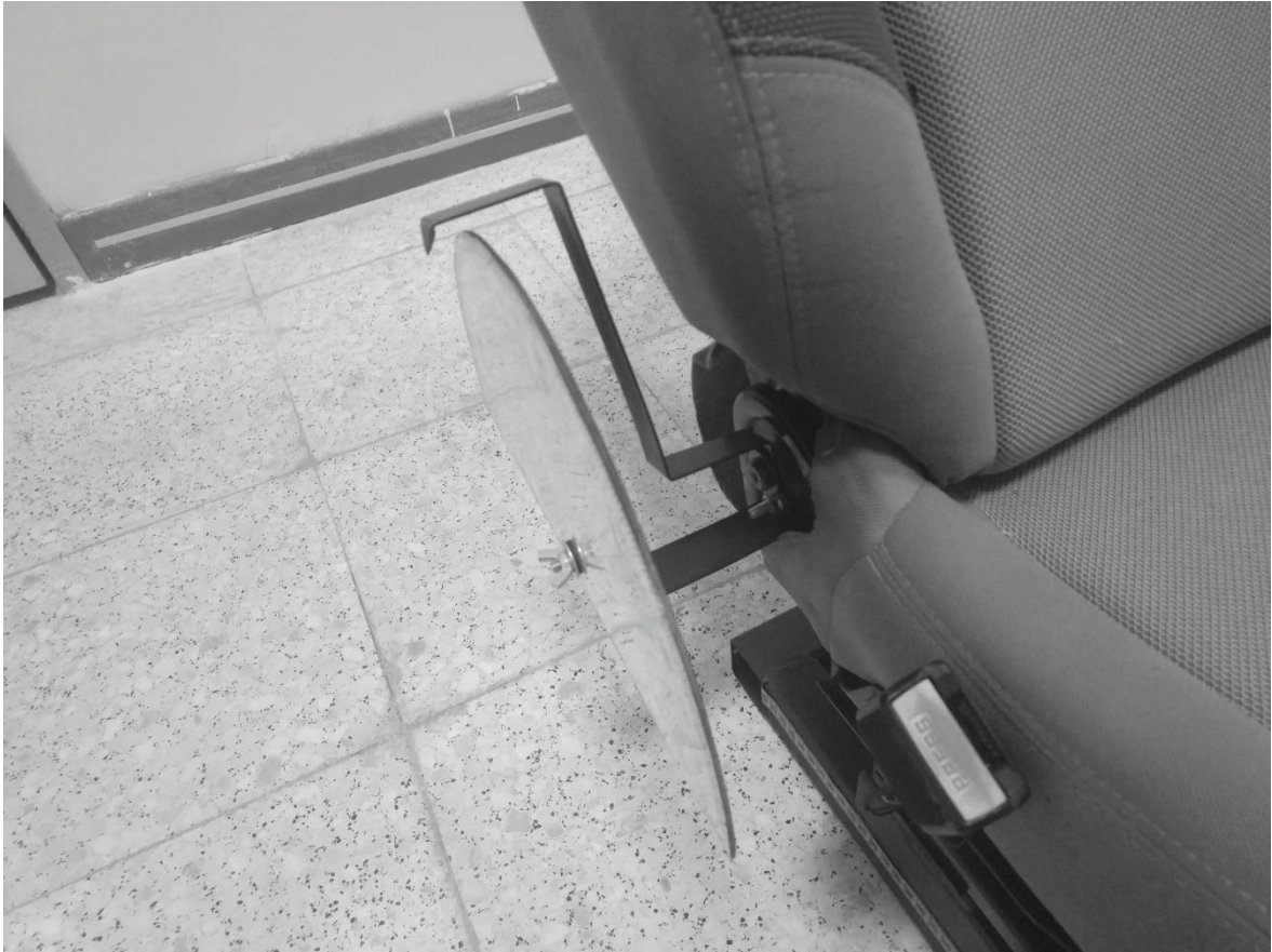
Figure 5 - Scale for seatback angle fixed on the seat's recliner
