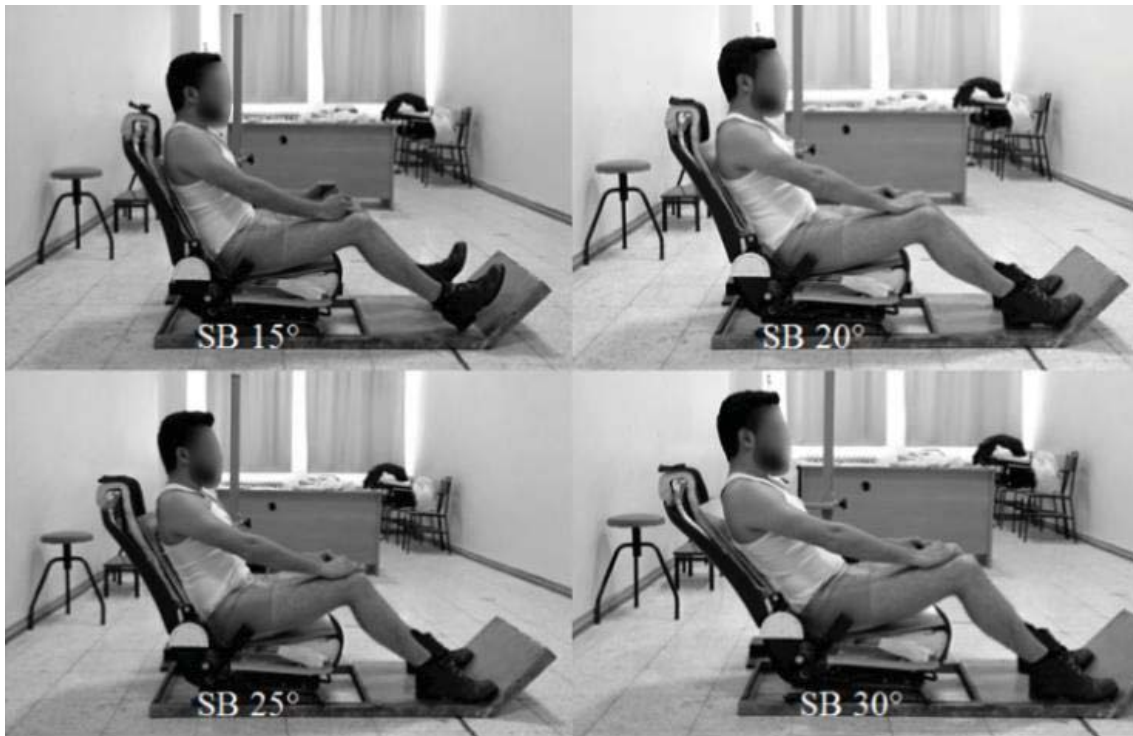
Figure 45 - Reference seating positions at various seatback angles
