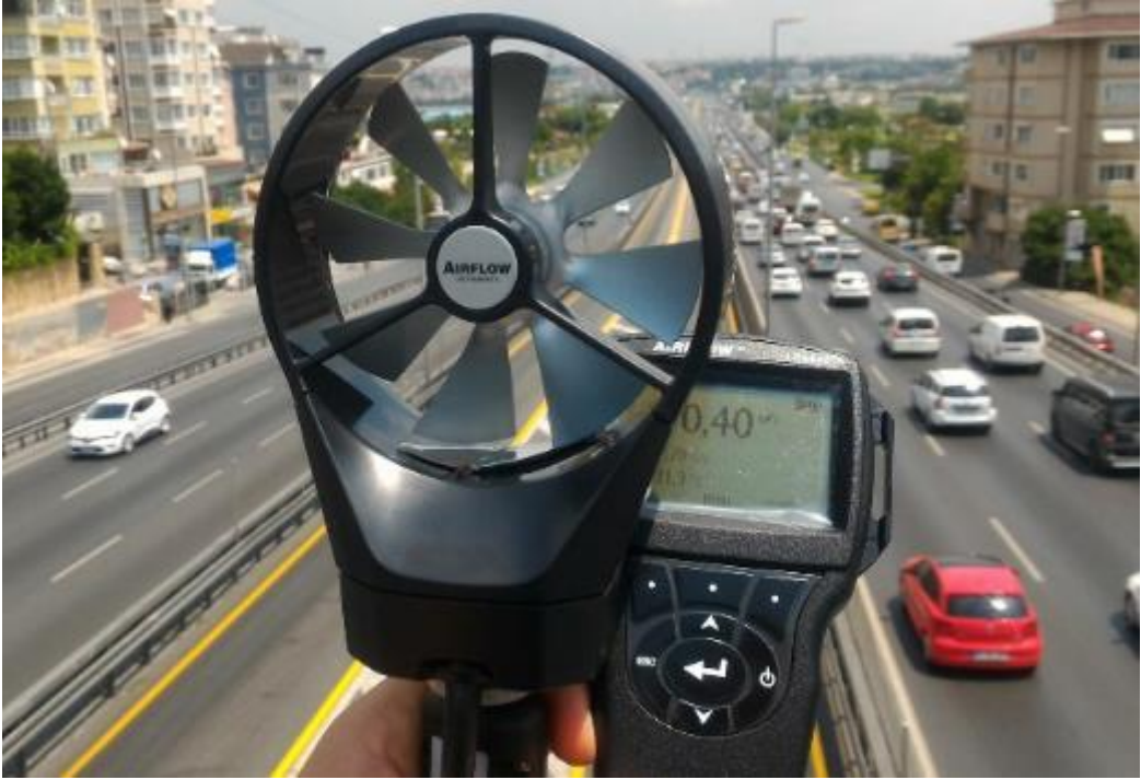
Figure 3-6 Wind speed measurement
