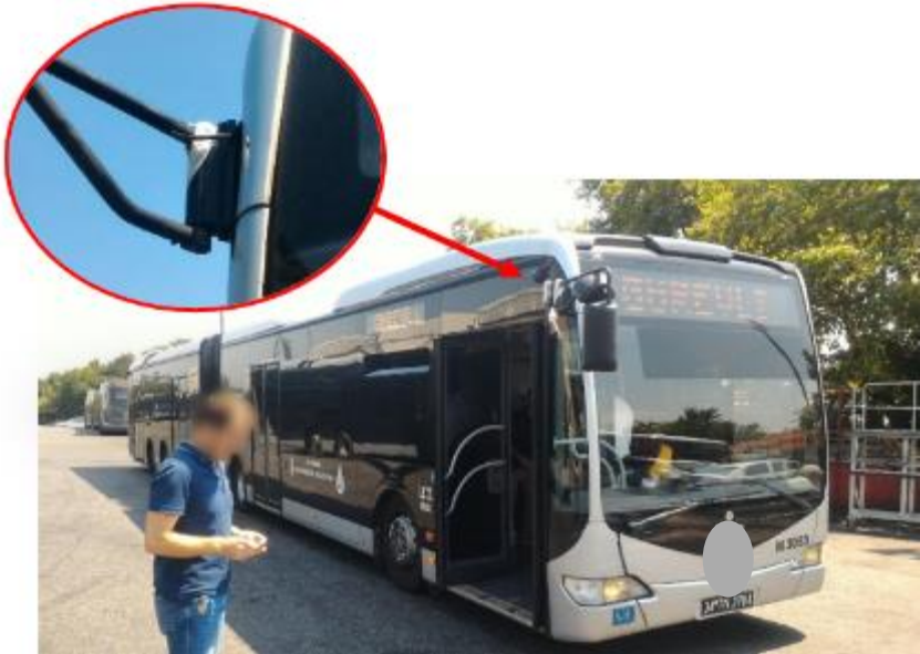
Figure 3-10 Position of the GPS antenna
