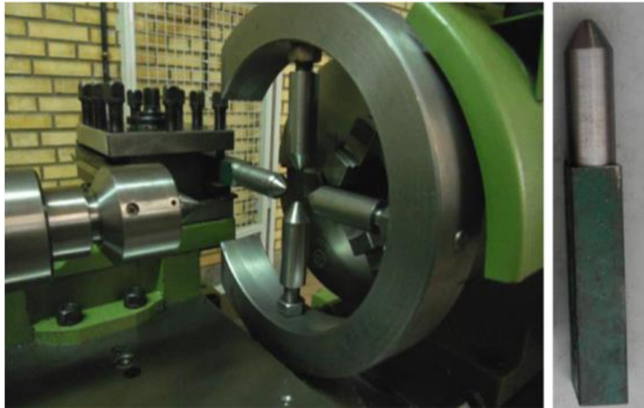
Figure 9 The Test Fixture and Rolling Tool [38]
