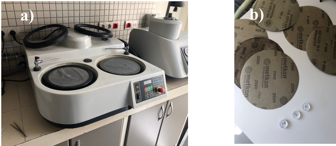
Figure 3.2 a) Metcon Forcipol 2P polishing station b) Silicon carbide paper of grid size 800, 1000 and 2500.
