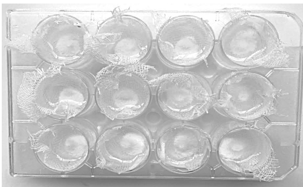
Figure 10. Image of sterile IBS samples in ultrapure water after 1 hour of incubation. B11(1), B11(2), B11(3), B12(1), B12(2), B12(3), B22(1), B22(2), B22(3), B21(1), B21(2) and B21(3) (from left to right)
