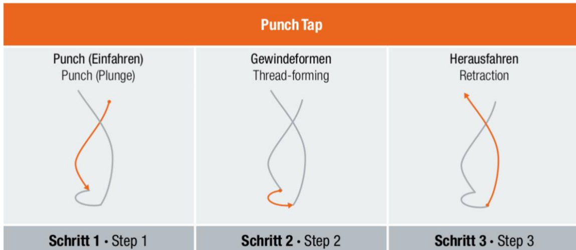
Figure 12 Working Mechanism of Punch Tap[13]
