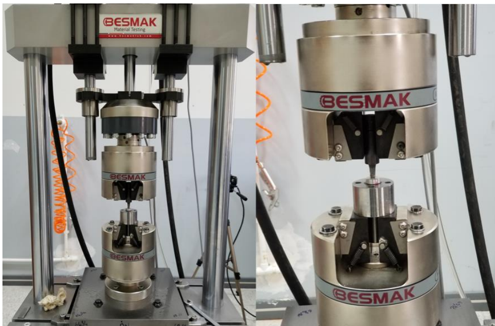
Figure 17 Test Setup for Mechanical Strength Measurement
