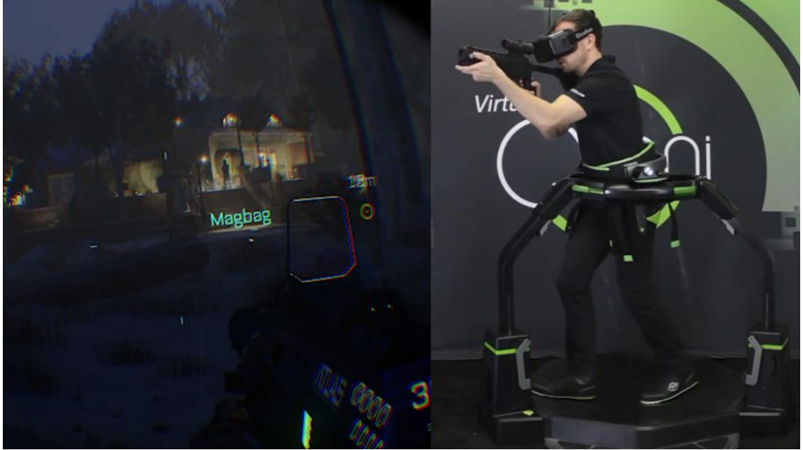
Figure 2: A man playing a video game using the locomotion simulator Virtuix Omni and the virtual reality headset Oculus Rift (right) and the game world as seen through his eyes (left). 6
