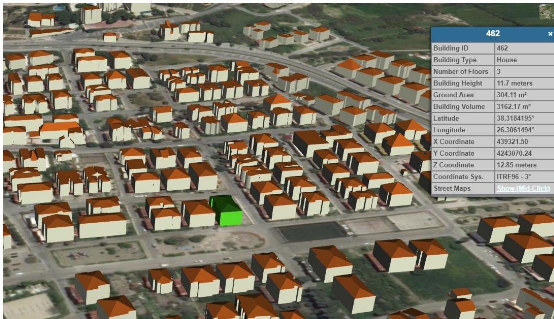
Figure 6.12 Showing selected untextured LoD2 buildings to attribute table on the customized web interface.
