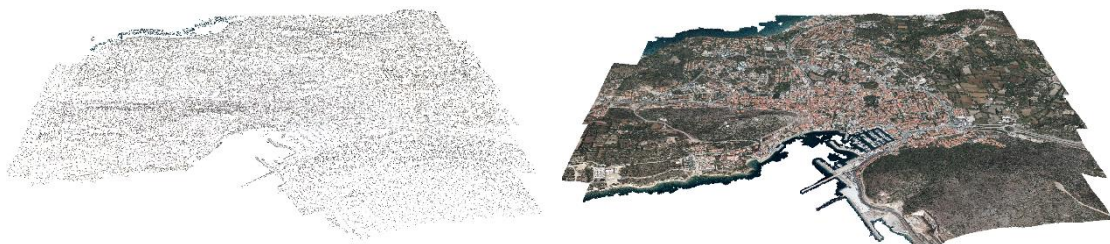
Figure 4.9 Generated Tie points (left) and dense point cloud (right)
