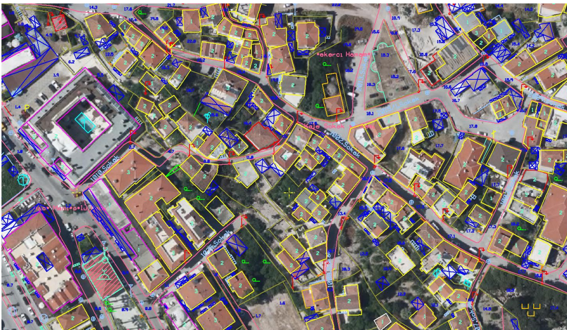
Figure 4.1 Manual feature extraction from stereo aerial images
