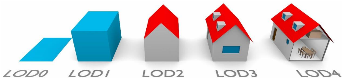
Figure 2.2 Levels of Detail in CityGML by Biljecki et al. [24]
