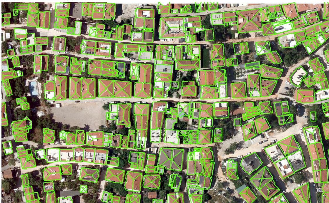
Figure 4.16 Automatically generated roof geometries overlaid on the orthophoto with 10 cm resolution.
