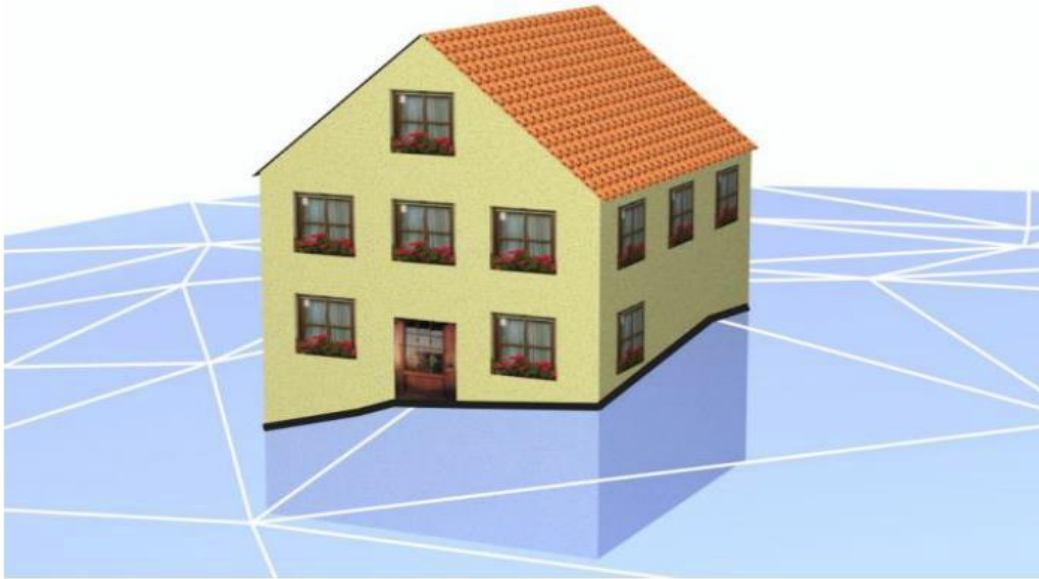
Figure 2.7 Example of the Terrain Intersection Curve represented as a black line [22].
