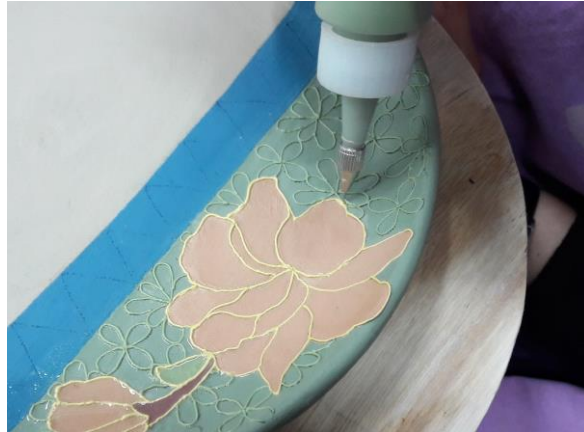
Figure 61: Slip trailing decoration process (Asmahazi Osmera, 2018)
