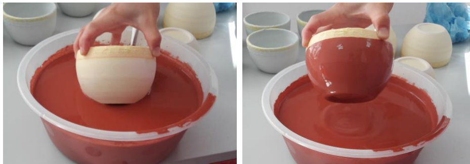
Figure 65: Glazing process (Asmahazi Osmera, 2018)
