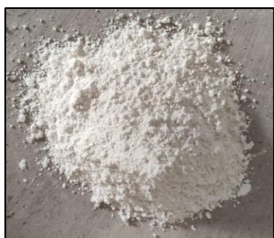
Figure 3.5. Digital camera image of \alpha -type hemihydrate
