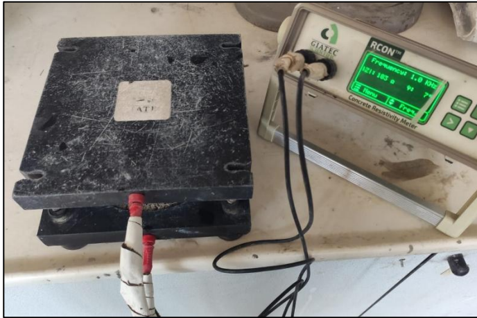
Figure 3.30. GIATEC RCON™ concrete electrical resistance measuring device
