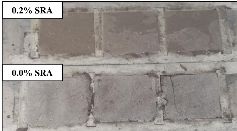
Figure 4.1. The effect of the setting retarder addition on the surface of mixtures
