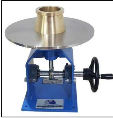
Figure 3.27. Representative images showing the details of the mini flow table test
