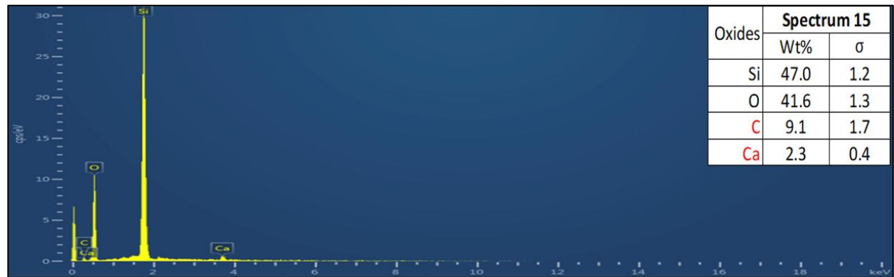
Figure 4.33. EDX analysis of CB26(1) composite with different spectrums
