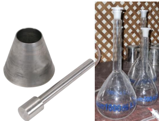
Figure 3.4 Cone/hammer used to control the SSD state of fine aggregate and pycnometer used for weight measurements
