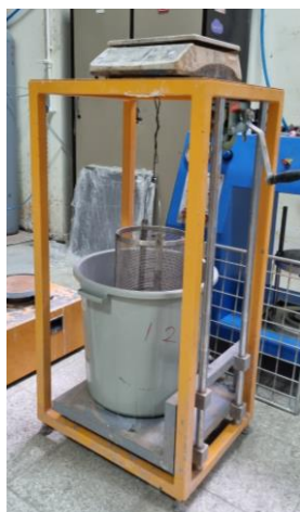
Figure 3.3 Water tank, wire basket and weight measuring device used to measure the weight of the aggregate in water
