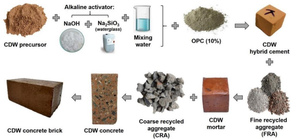
Figure 2.10 The process of evaluating CDW as a binder using the alkali activation method (Robayo- Salazar et al., 2020)
