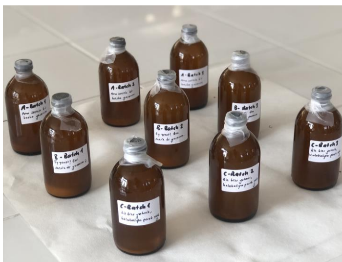
Figure 3.4. Used batch reactors during the anoxic period in the determination of the form of urease enzyme test (Table 3.2)
