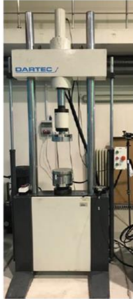
Figure 3.7 DARTEC Uniaxial Compression Machine
