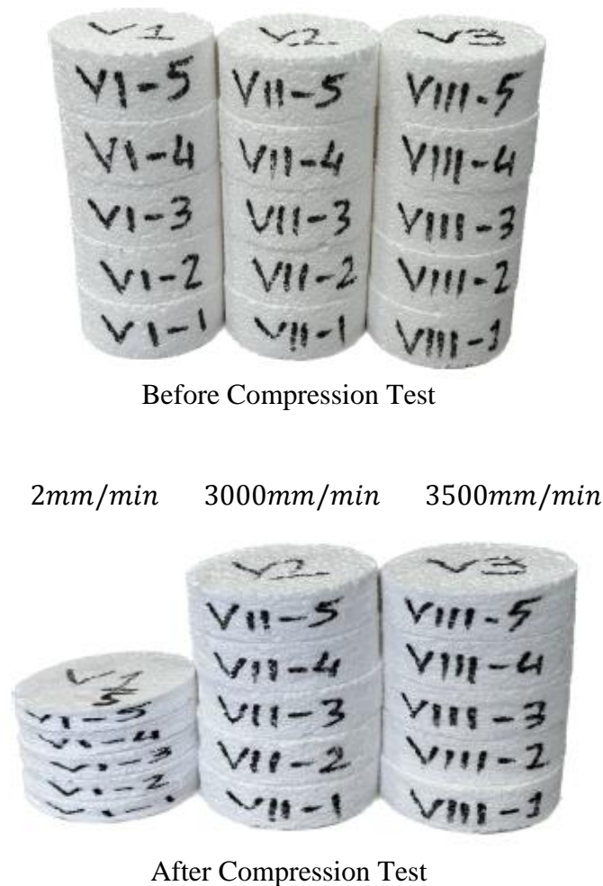
Figure 4.2 Foam specimens before and after the uniaxial compression test
