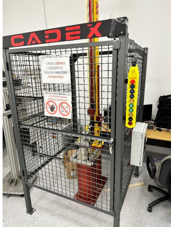
Figure 5.1 CADEX Monorail Impact Setup
