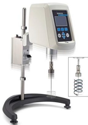
Figure 3.8. Brookfield DV2T Extra viscometer [118]
