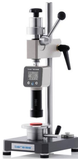
Figure 3.10 Shore A hardness durometer (BS61 II, Bareiss, UK)
