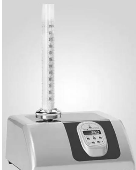
Figure 3.2. J. Jolting volumeter (Jolting Volumeter Type STAV II, J. Engelsmann AG, Deutschland) setup for measurement of tapped density
