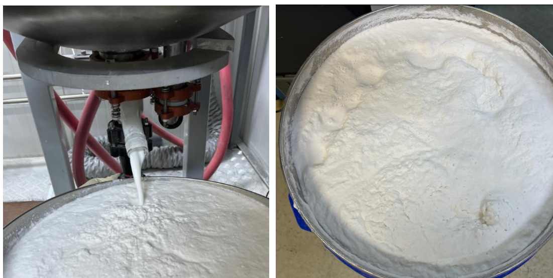
Figure 3.6. IDP-coated HMX collected on a sieve before drying
