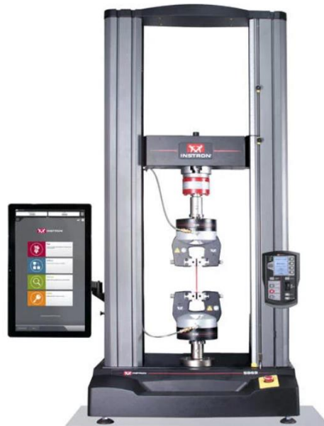
Figure 3.11. Universal Testing Instrument (5900 Series, INSTRON, US)
