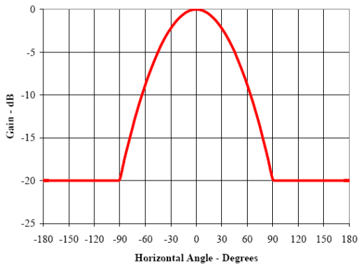
Figure 1.5. Simplified antenna pattern [ITU-R M.2135].
