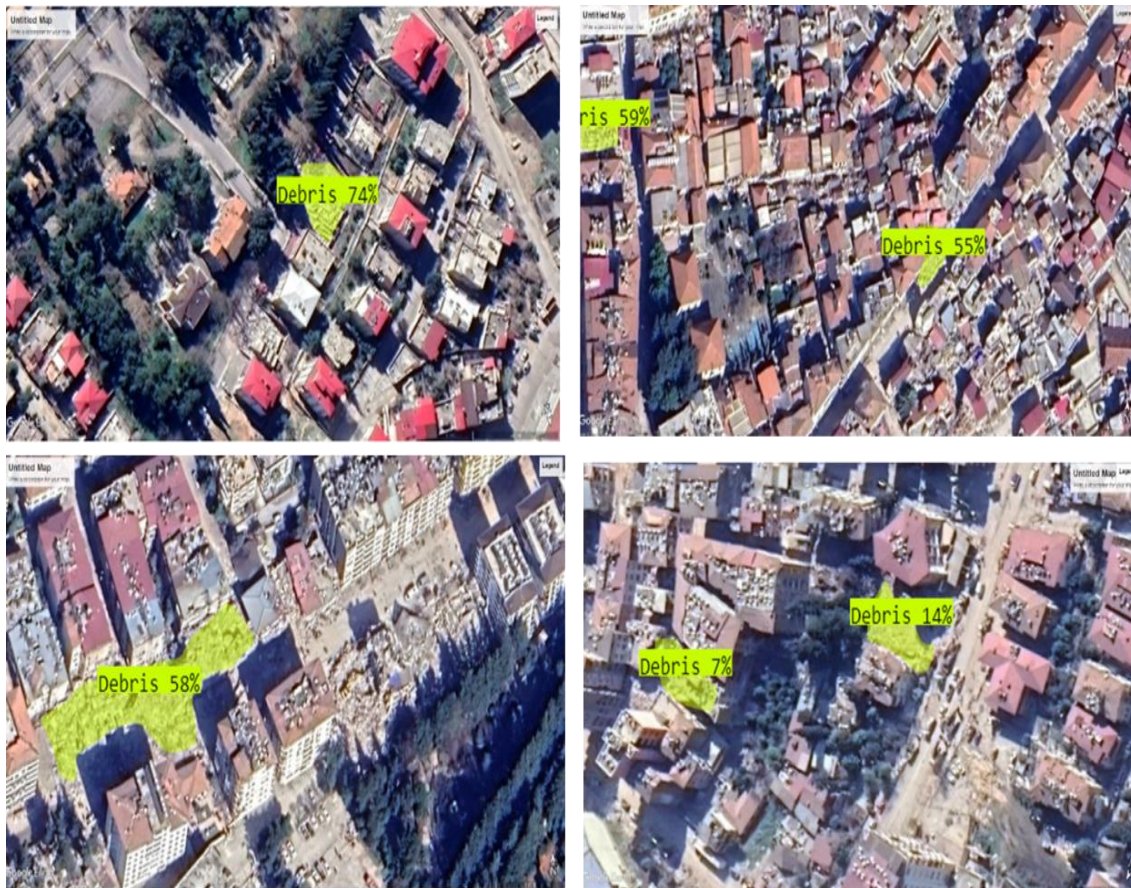
Figure 3.49 A Visual Overview of satellite Dataset Analysis of Roboflow Instance Segmentation Results
