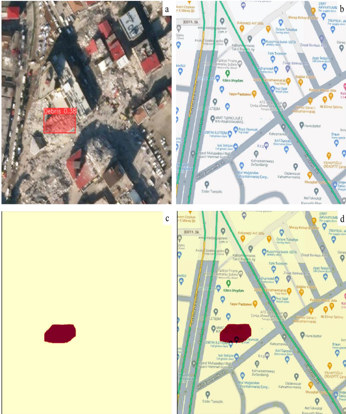
Figure 0.56 a) YOLOv8 Predicted Debris Result for Coordinates 316895.3, 4161318, b) Associated Traffic Map, c) Mask Representation, d) Overlay of Mask and Traffic
