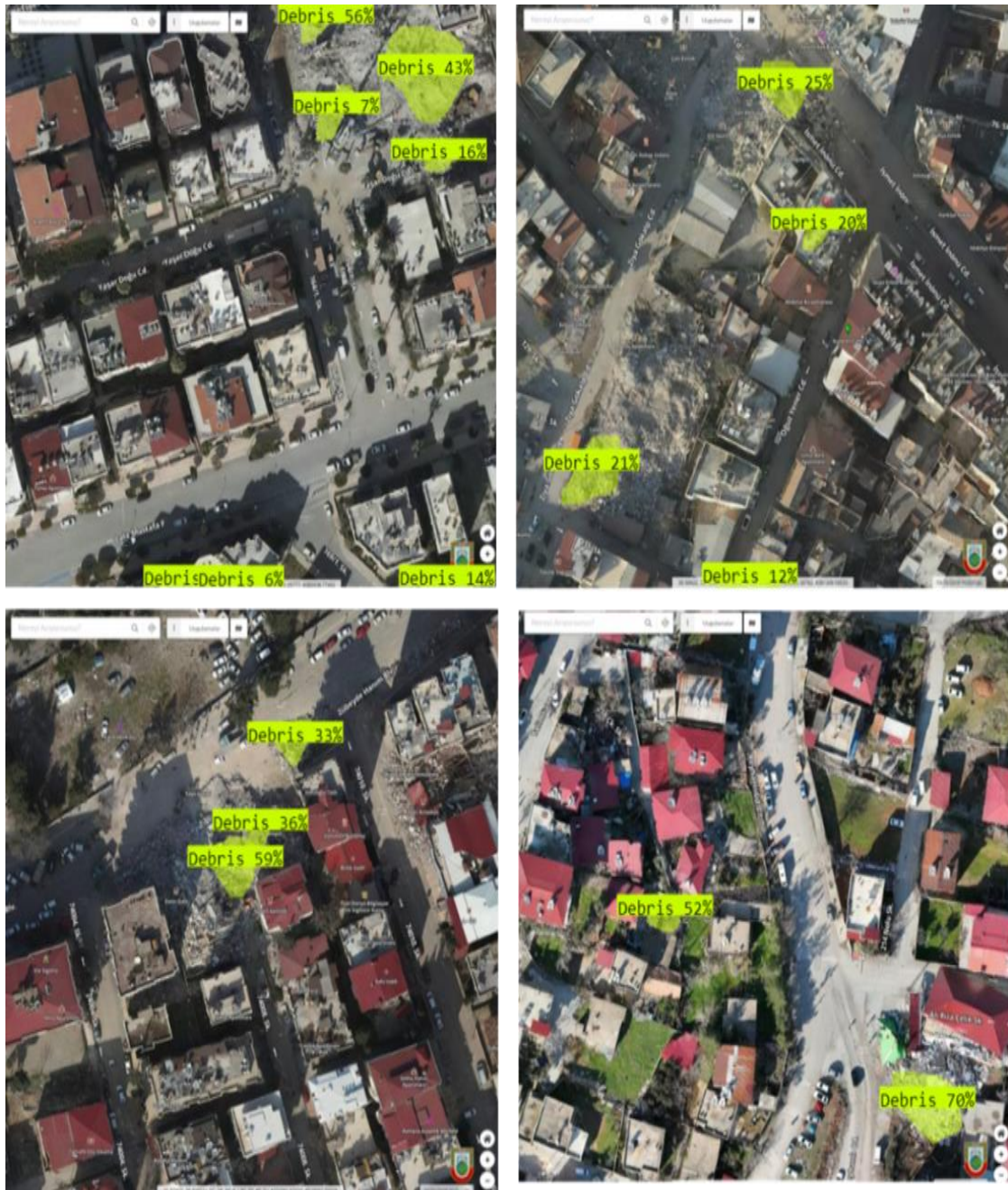
Figure 3.50 A Visual Overview of drone based Dataset Analysis of Roboflow Instance Segmentation Results
