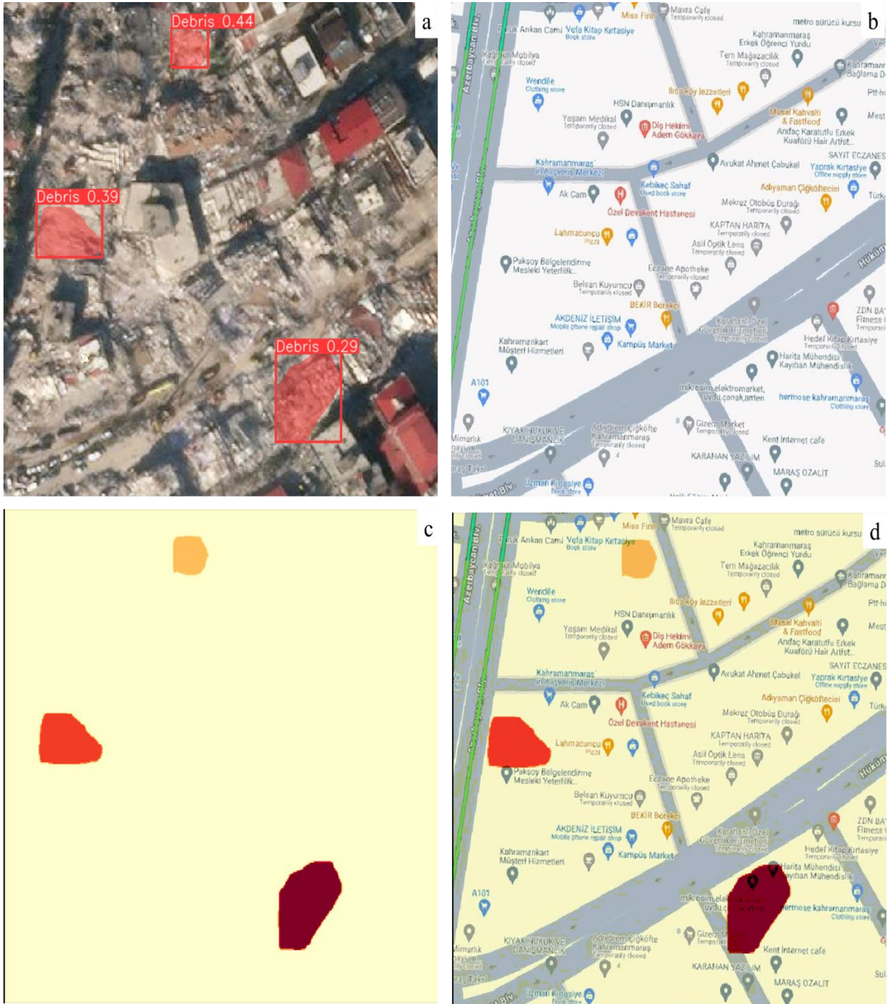
Figure 0.55 a) YOLOv8 Predicted Debris Result for Coordinates 316877.6, 4161036.4, b) Associated Traffic Map, c) Mask Representation, d) Overlay of Mask and Traffic
