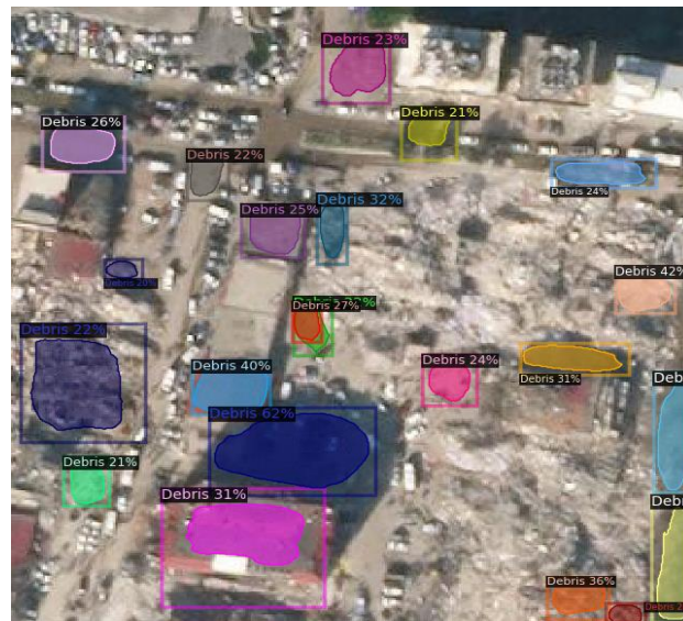
Figure 3.46 Test Data Predictions Utilizing Mask R-CNN via Detectron2 with 8 Epochs and 2000 Iterations
