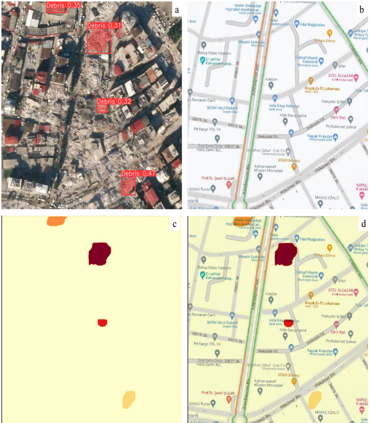
Figure 0.53 a) YOLOv8 Predicted Debris Result for Coordinates 316717.3, 4161155, b) Associated Traffic Map, c) Mask Representation, d) Overlay of Mask and Traffic
