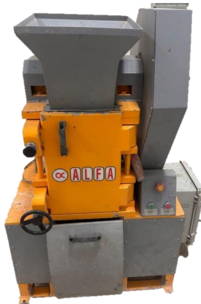
Figure 3.1 Laboratory type jaw-crusher which is utilized to decrease the maximum grain size to 2mm
