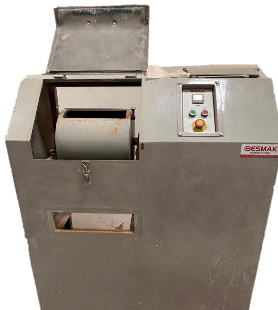
Figure 3.8 Laboratory type ball mill which is used to grind brick waste material
