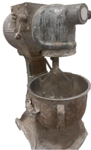
Figure 3.10 Mixer which is used to prepare mortar
