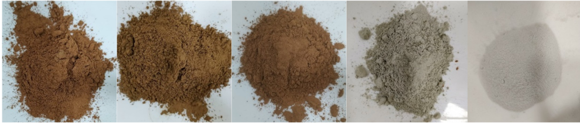
Fig. 2.1. Powderized CDW-based materials (left to right: RT, RCB, HB, C, and G)
