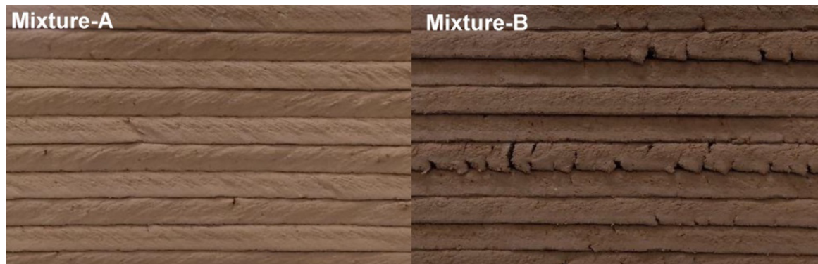
Fig. 1.10. Visuals of multi-layer specimens of 3D printed geopolymer mixtures. Mixture A is characterized by a low viscosity, whereas Mixture B exhibits a high viscosity profile [97]
