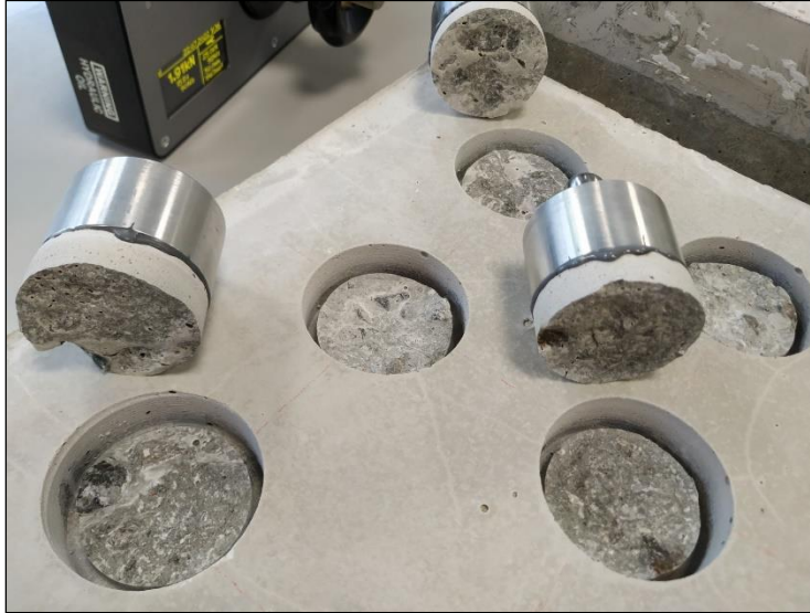
Figure 4.55. Samples that broke off as a result of the test on the 28 th day in the sample with a thickness of 2 cm
