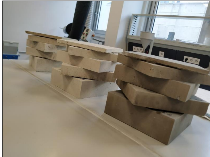
Figure 3.20. Samples with a thickness of 10, 20, 30, 40, 50 mm
