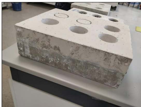
Figure 3.27. Substrate concrete sample with 5 cm thickness PCM(6)CF(0.1) coded composite
