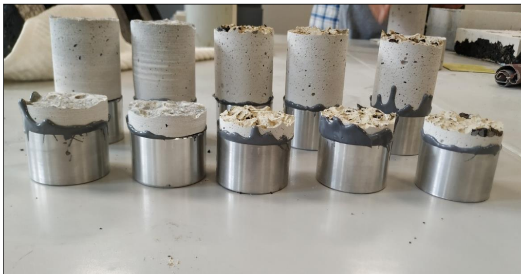
Figure 4.54. The rupture patterns formed on the 28 th day in 1 cm and 5 cm samples
