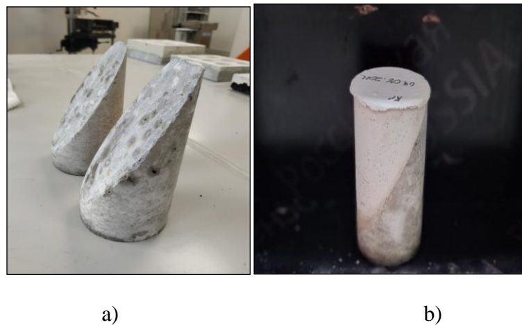
Figure 3.23. a) Substrate concrete samples cut at an angle of 30 °C b) Monolithic state of PCM(6)CF(0.1) mixture and substrate concrete sample
