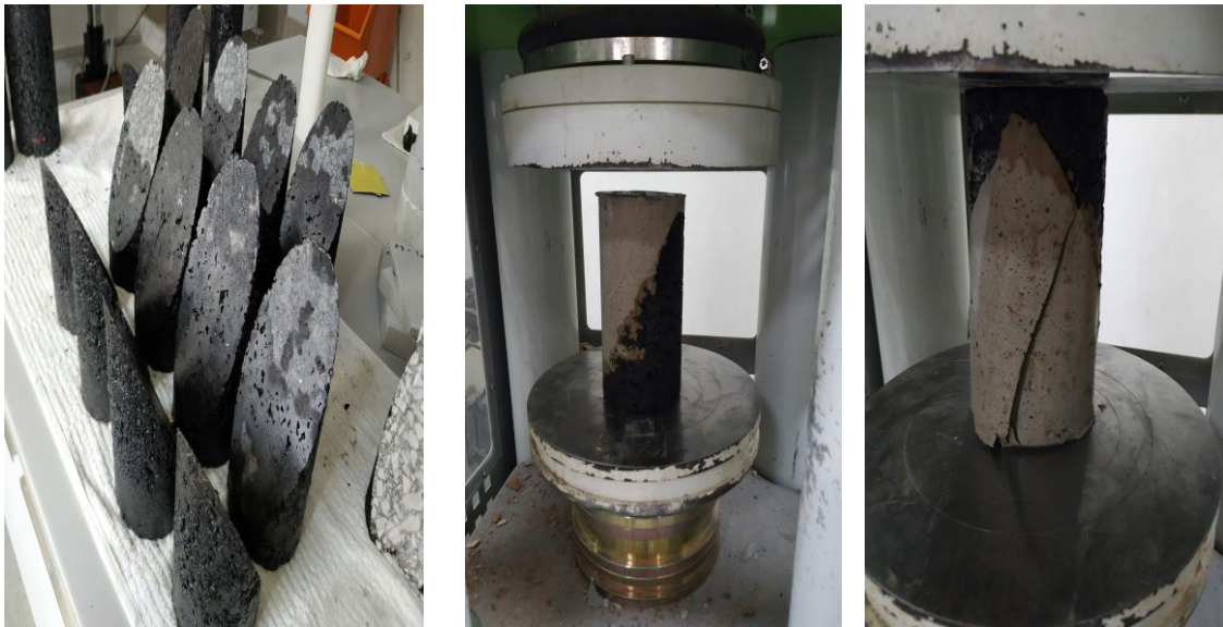
Figure 4.52. Stages of slant shear test
