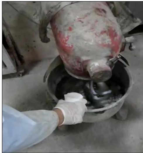
Figure 3.11. Addition of PCM dispersion to the mortar mix
