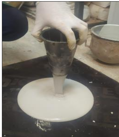
Figure 3.13. Determination of the consistency of mixtures with the mini slump flow spread test
