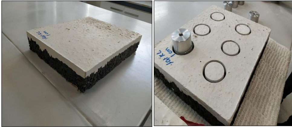
Figure 3.28. a) 1 cm thick PCM(6)CF(0.1) coded composite and substrate asphalt sample b) Core taken and metal ring attached sample
