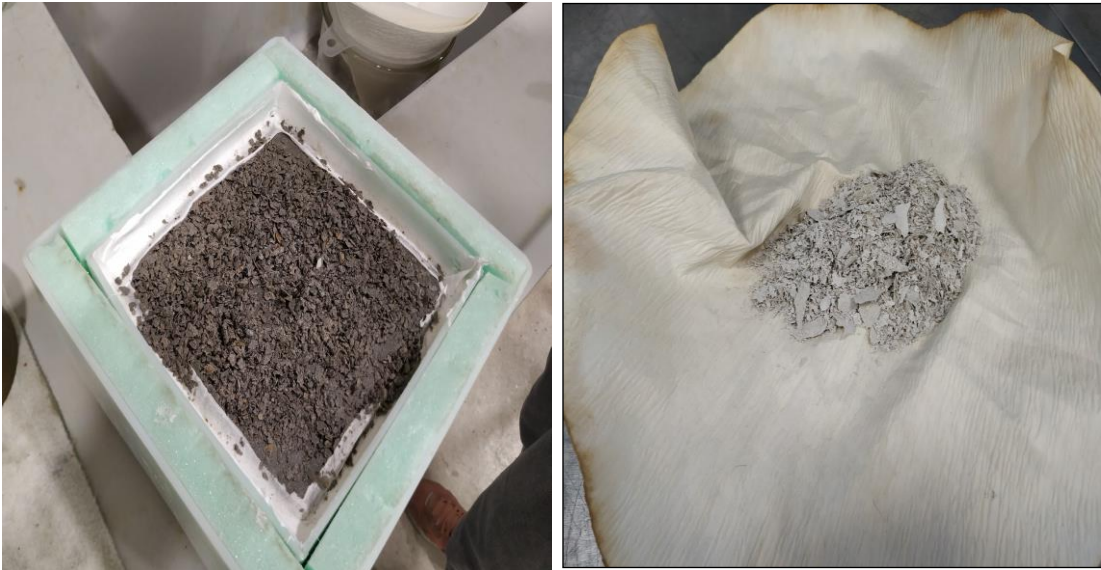
Figure 4.51. The spalling material from the PCM(6)CF(0.3) coded composite
