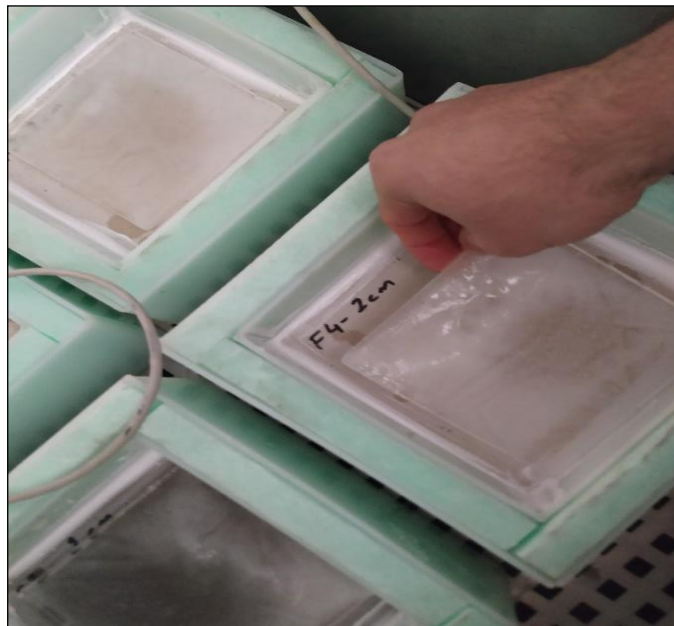
Figure 3.21. The process of placing ice on the samples in the cabinet
