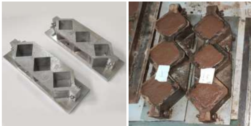
Figure 3.14. 50 \times 50 \times 50 mm 3 empty and poured cubic molds.
