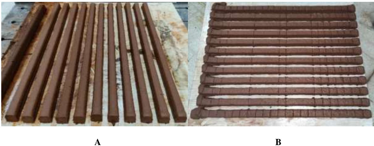
Figure 3.17. The preparation of the specimens involved (A) utilizing two-ply filaments and (B) cutting fresh filaments.
