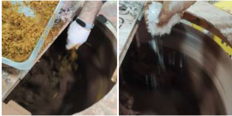
Figure 3.13. Adding WFF– Polypropylene (PP) fiber to mixture.
