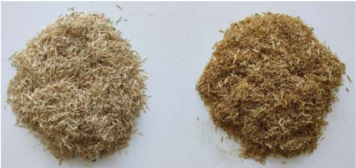
Figure 3.24. Untreated WWF and the WWF treated with alkali.
