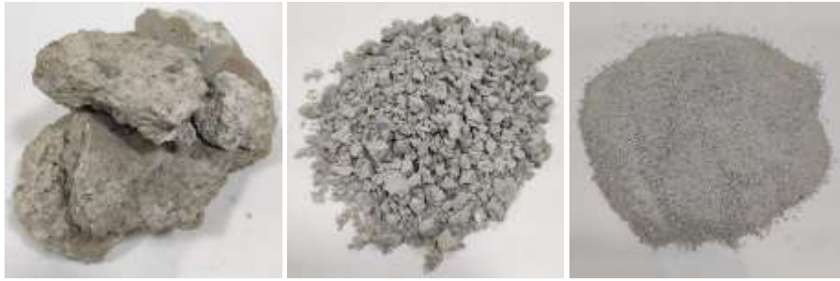
Figure 3.10. From left to right, the raw, crushed, and grinding phases of the RCA.
