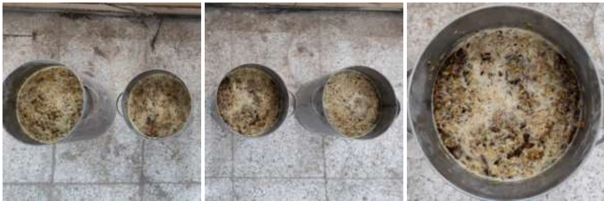
Figure 3.23. Process of immersing WWFs in an alkali solution.
