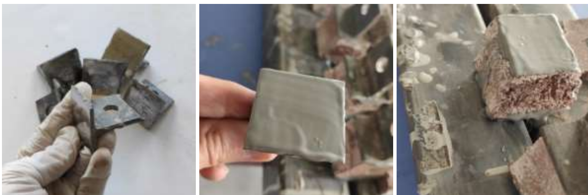
Figure 3.21. From left to right, T-shaped metal profile, glued profile, glued sample.
