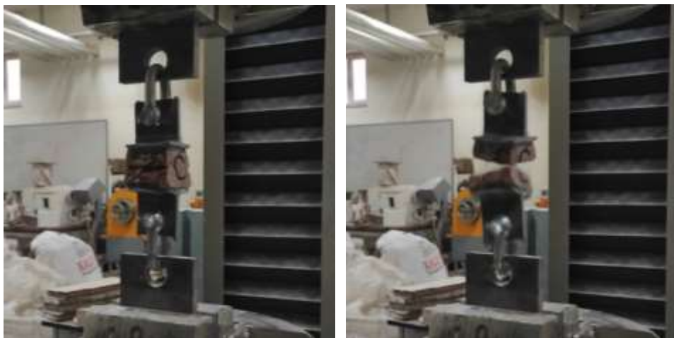
Figure 3.22. Sample subjected to direct tensile stress.
