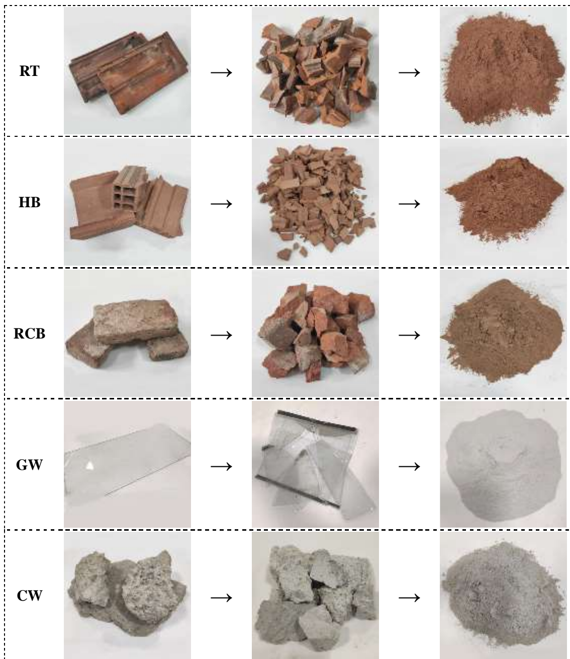
Figure 3.3. Raw, crushed, and grinding phases of the CDW materials.
