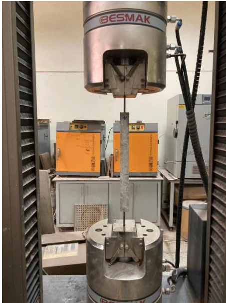
Figure 3.6 Creation of cracks with various widths via uniaxial tension.
