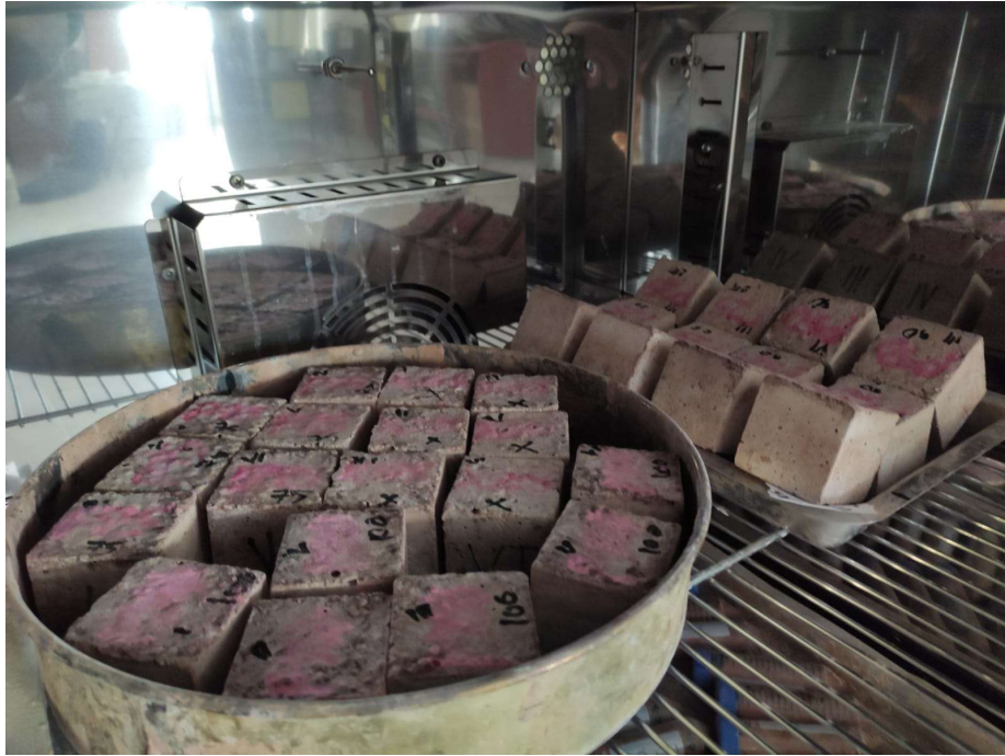
Figure 3.24 The geopolymer samples placed in an oven to dry
