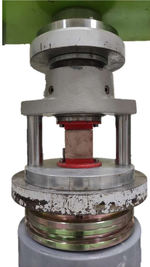
Figure 3.23 Representative image of compressive testing of the specimens
