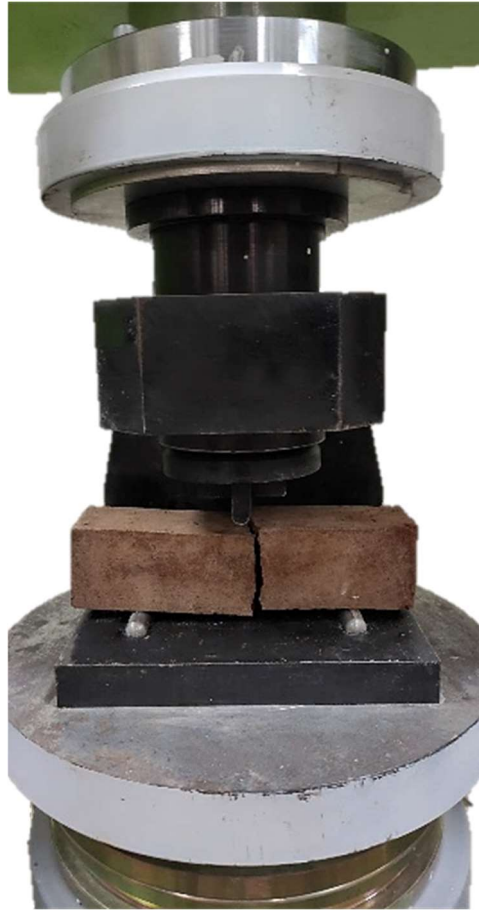
Figure 3.22 Representative image of flexural testing of the specimens
