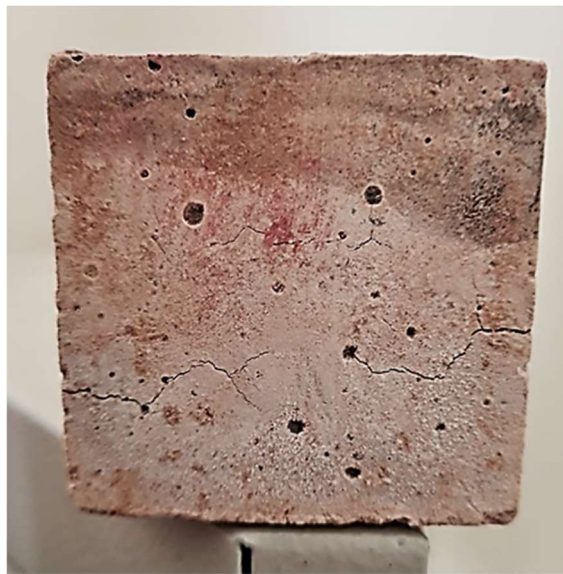
Figure 4.8 Illustration of the surface cracks
