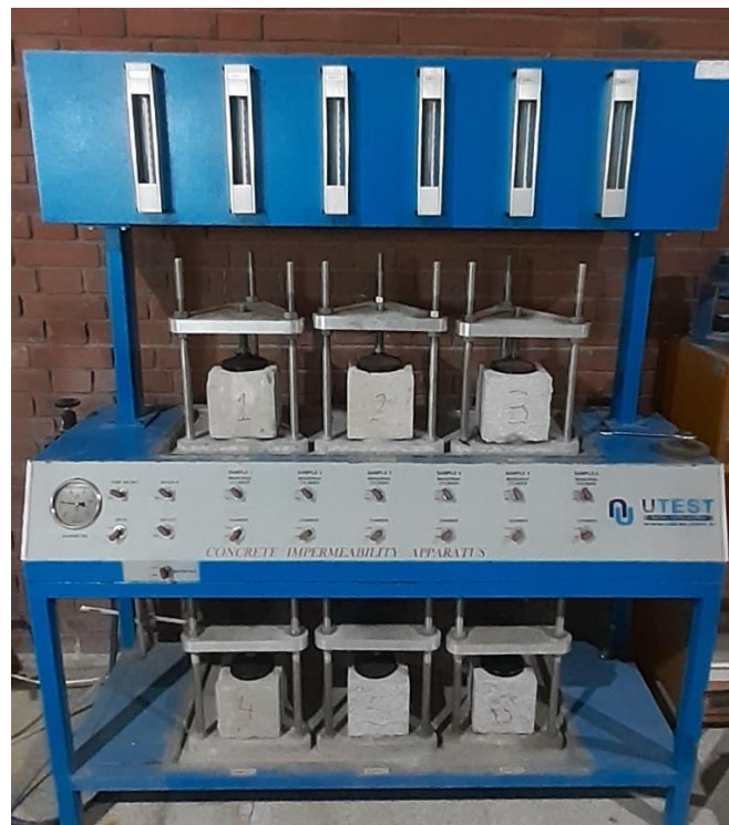
Figure 4. 1. Pressurized water experiment setup
