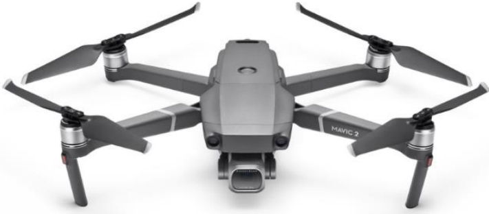
Figure 19. Drone used to collect images (DJI Mavic 2 Pro)
