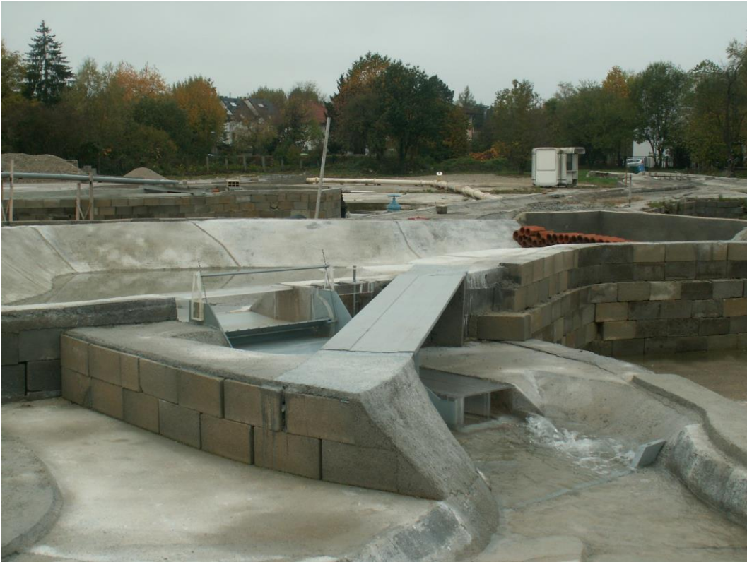
Figure 2.6 Physical model of Suša Dam built at the University of Ljubljana (Photo was taken during a technical study visit at 26/10/2022)
