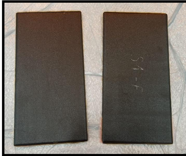
Figure 3.16. Demolded samples (Base & Fiber configurations)
