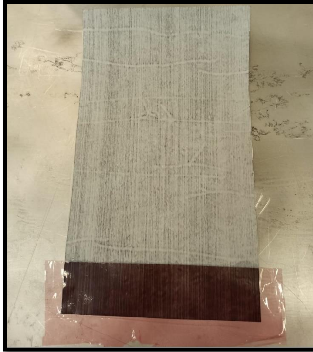
Figure 4.11 Result of veil removal process with titanium collector
