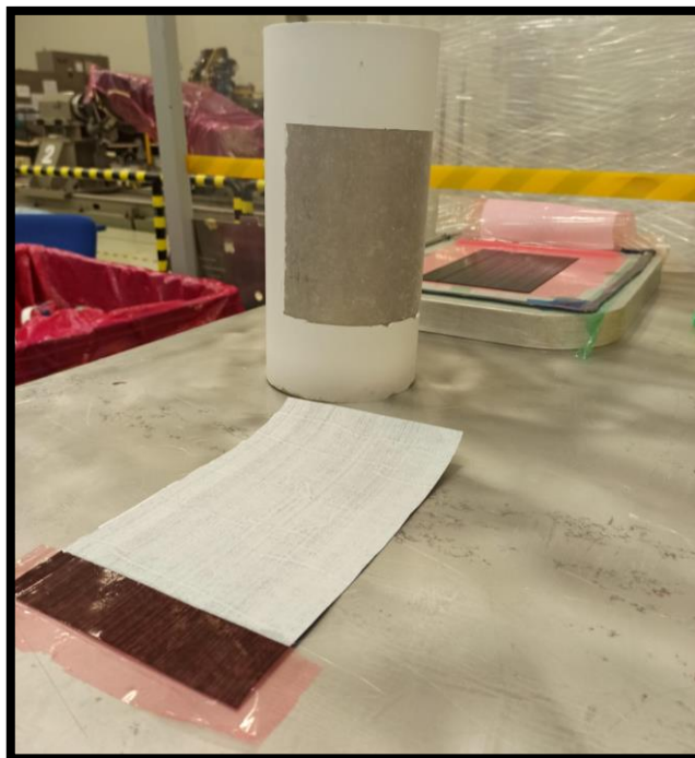
Figure 3.13. Separation of fiber adhered UD from titanium collector
