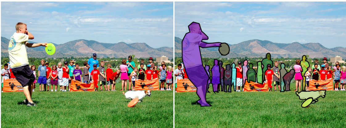
Figure 2.2 Semantic segmentation of pixels translates to understanding the correct labels of visual data. On the left, the original image is taken from the MSCOCO dataset [11], and on the right semantic annotations are drawn onto the same image.
