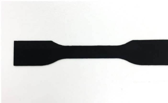
Figure 3.70. Specimen prepared with Universal ISO-37.1 die cutter for tensile tests
