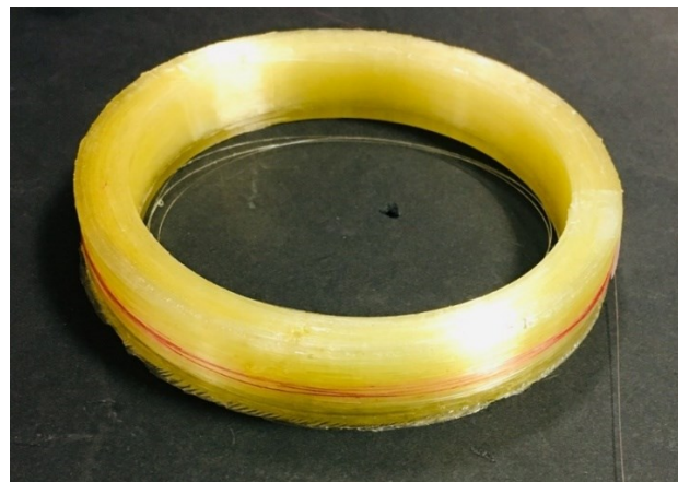
Figure 4.8. Free standing fiber optic coil
