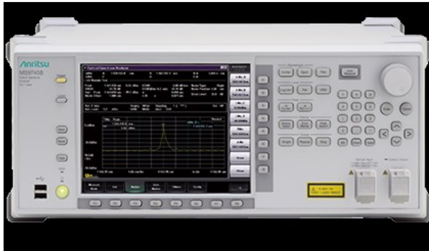
Figure 3.13. Picture of optical spectrum analyzer (OSA) used for optical spectrum measurements
