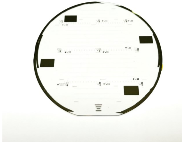
Figure 3.48. LiNbO3 wafer after Ti-etch
