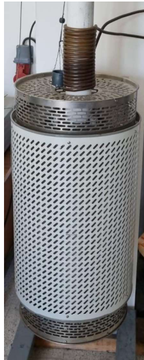
Figure 3.2-1. Vertical Cylindrical Furnace.
