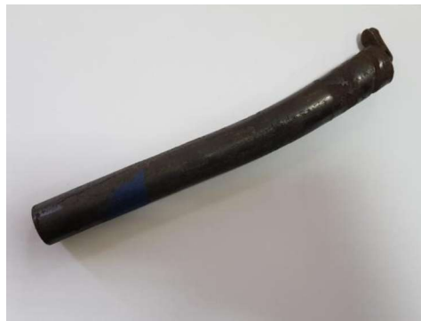
Figure 3.1-1. Hot extruded bulk \text{Ni}_{50}\text{Ti}_{30}\text{Hf}_{20} (at.%) alloy [17].
