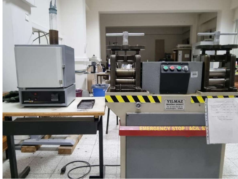
Figure 3.4-1. Cubic furnace and laboratory sized rolling setup.
