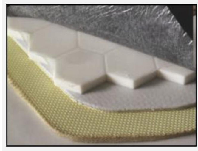
Figure 2. 6. A ceramic armor with an aramid-based composite backing plate [9]
