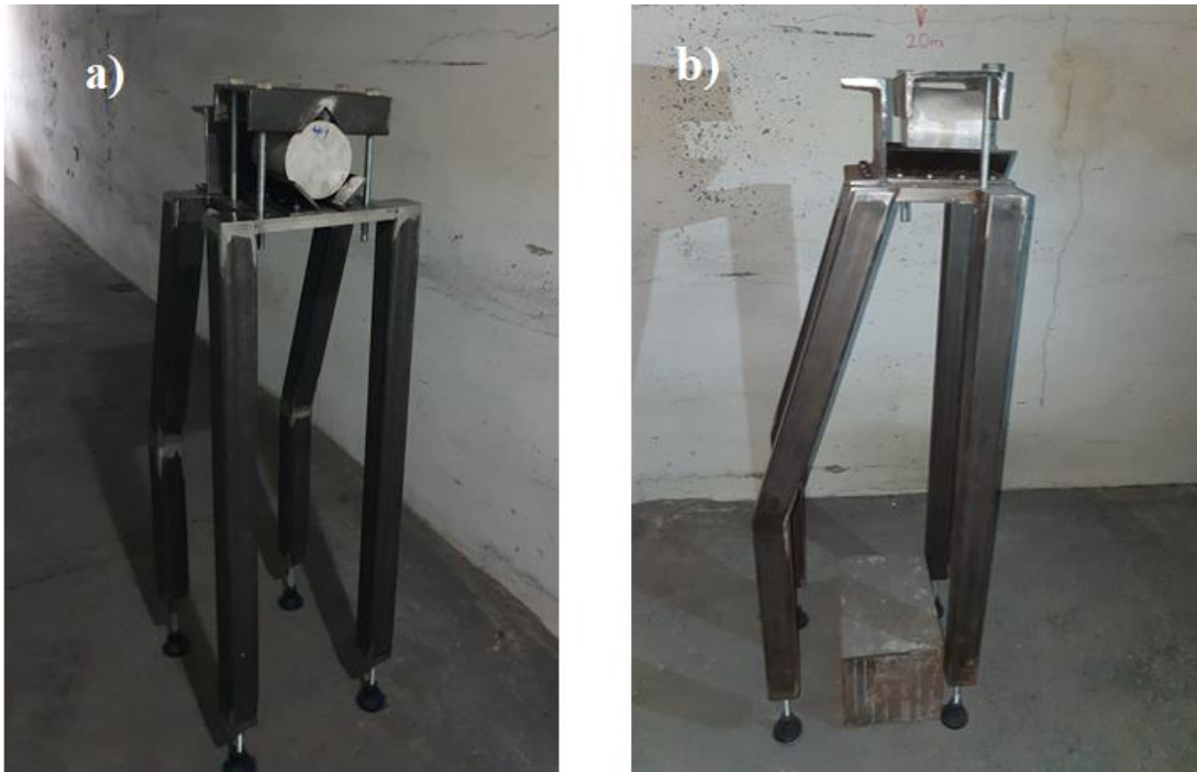
Figure 4. 4. Target carrier stand with cylindrical block a) isometric view, b) side view
