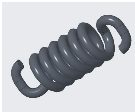
Figure 34 - 3D Model of Tension Spring (6)
