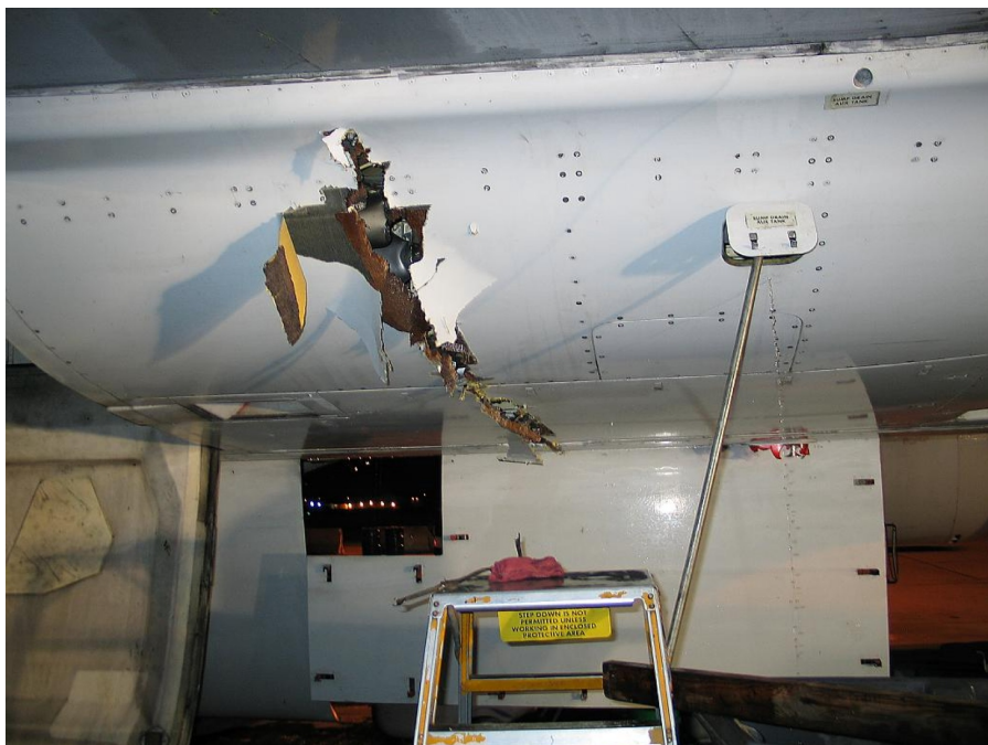
Figure 1.6 Burst Failure and Aftermath
