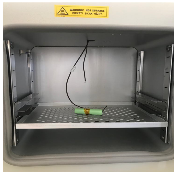
Figure 5.7. Thermal abuse testing system of a Li-ion cell that was placed in an oven.
