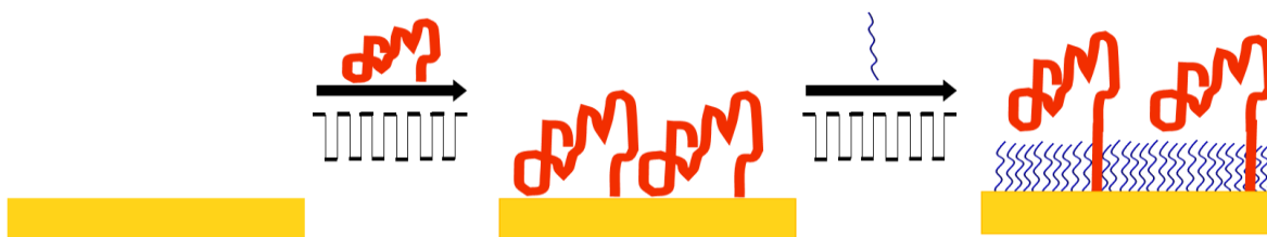
Figure 4.14. Schematic representation of the DNA sensor fabrication using the potential assisted immobilization method.
