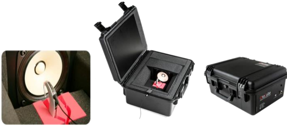
Figure 3.1. Portable desktop box (Otocube) used in audiometric examinations of CI users.
