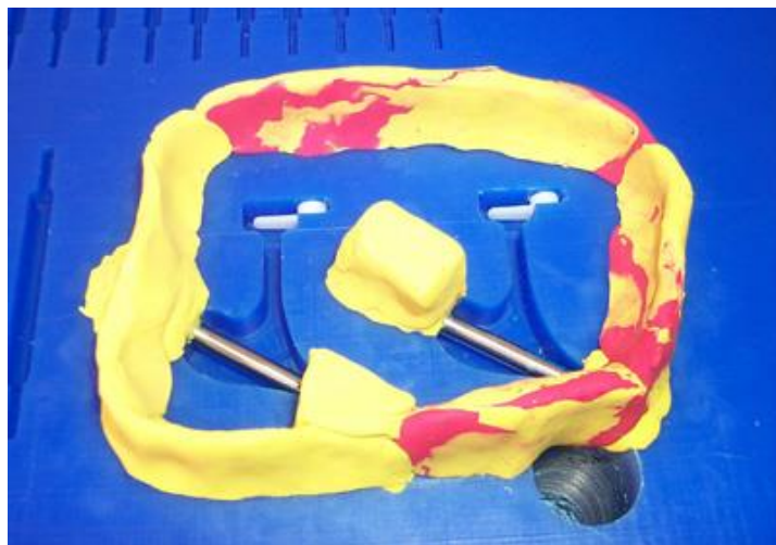
Figure 2.12. Sacrificial material (yellow), support material (blue) and embedded components [29]
