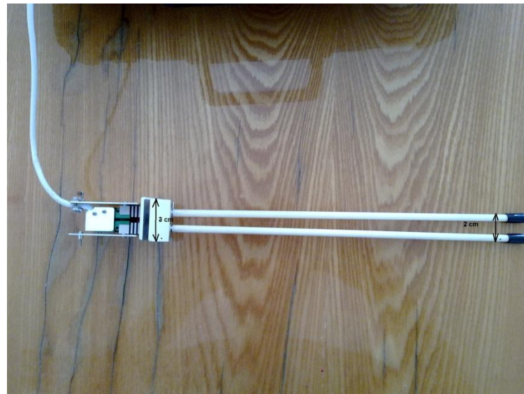
Figure 3.11 The Epsilon 3448 high temperature extensometer
