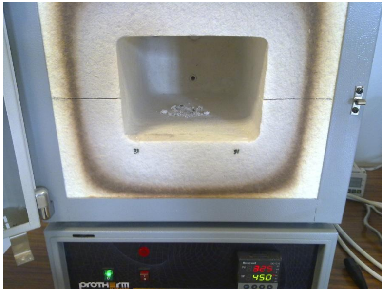
Figure 4.24 Vaporized AZ91 sample which was tried to be homogenized at 450C for 30 Minutes
