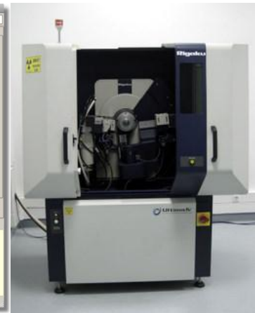
Figure 3.10 a) Match! Crystal Impact software b) Rigaku Ultima IV XRD device
