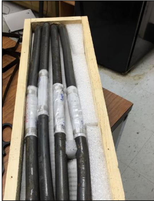
Figure 3.1-2 As Received 50Ni25Ti25Hf (at %) alloy extruded rods [1]
