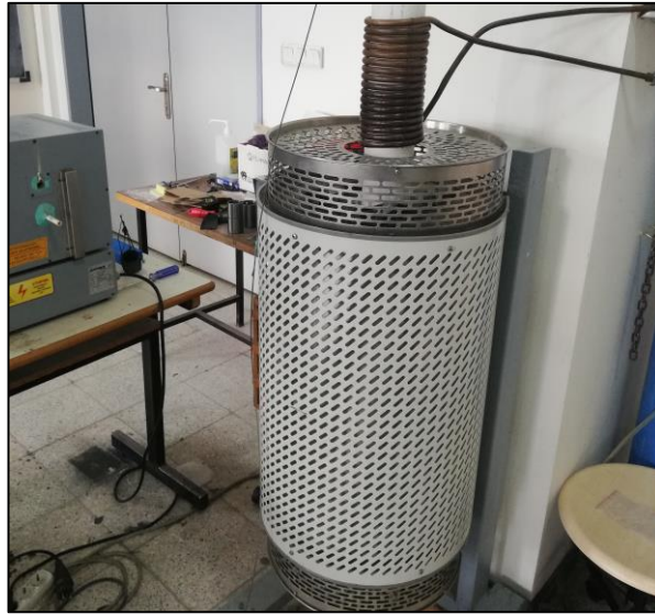
Figure 3.5-1 Vertical Cylindrical Furnace
