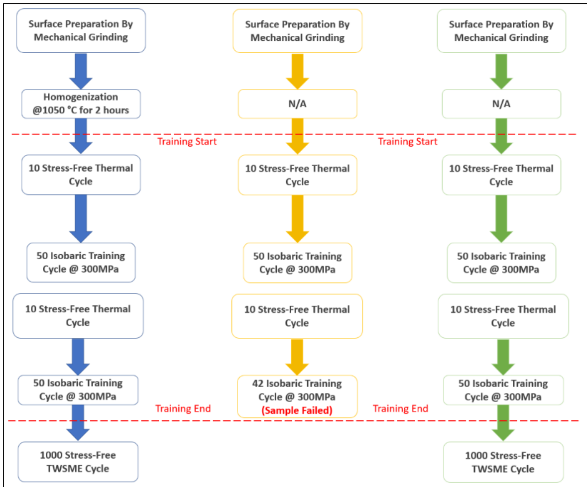
Figure 3.7-3 Entire Experiment Sequence-2 (including 1000 Stress-Free TWSME cycles)
