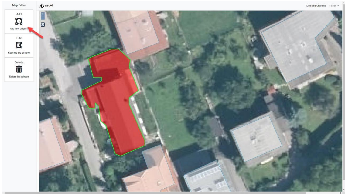
Figure 4.23. Adding detected building polygon to the user provided vector data (Can et al., 2021).
