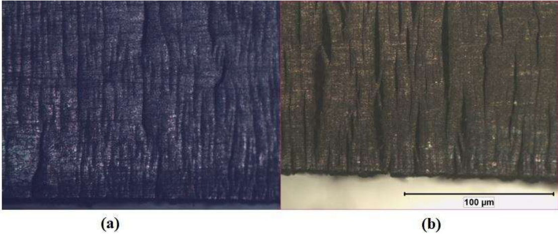
Figure 4.2-6. Optical Images H-WR2-500 Sample, which were taken at the end of, (a) 50 th Cycle (b) 110 th Cycle (Last Cycle).
