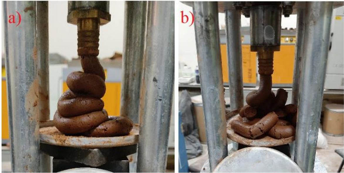
Figure 4.1 Representative images of extruded mixtures: a) continuously extruded, b) discontinuously extruded.
