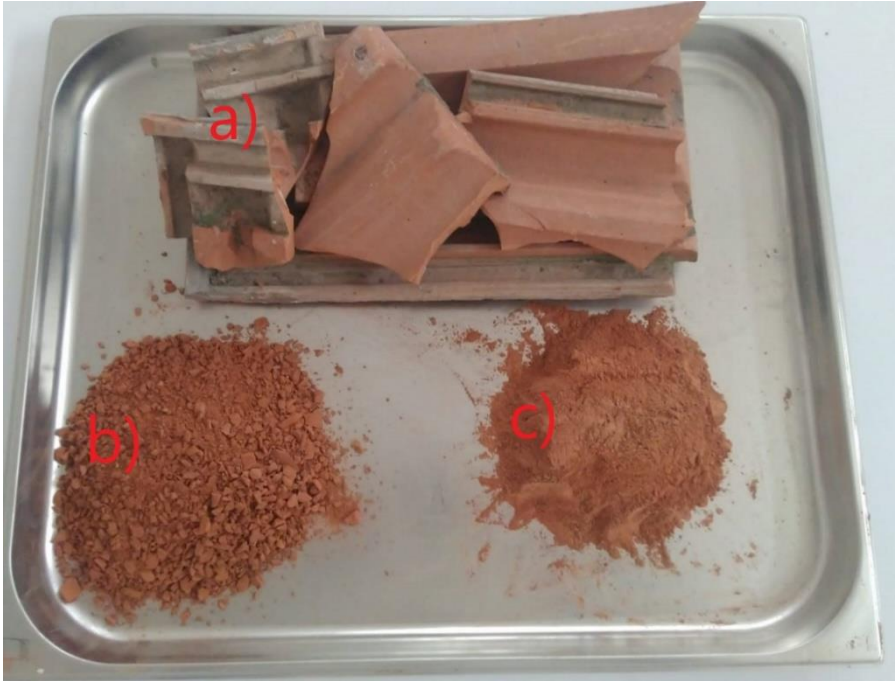
Figure 3.5 Crushing and grinding process of RT. a) Raw form, b) Crushed form, c) Ground form
