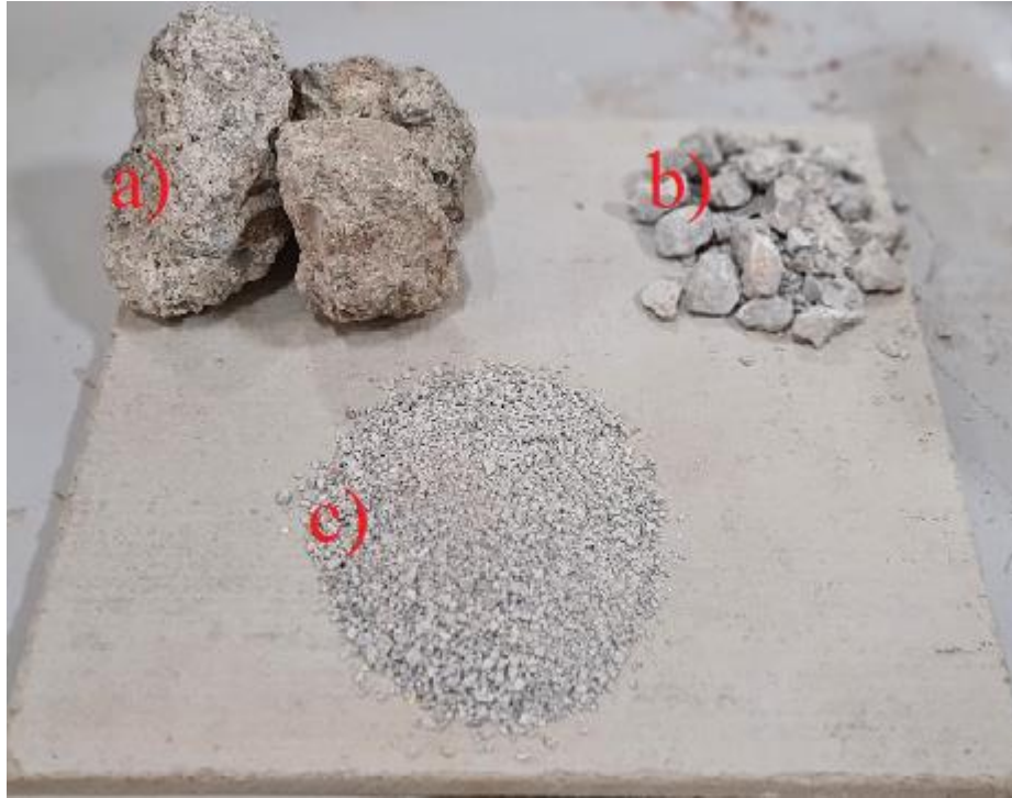
Figure 3.13 Detailed images of RCA a) raw form, b) crushed form, c) sieved form
