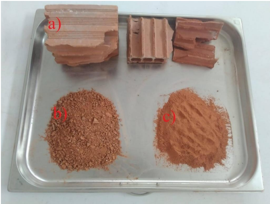
Figure 3.3 Crushing and grinding process of HB. a) Raw form, b) Crushed form, c) Ground form
