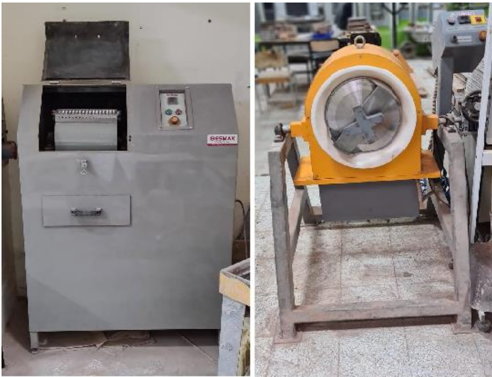
Figure 3.2 Representative images of different types of ball mills used in study
