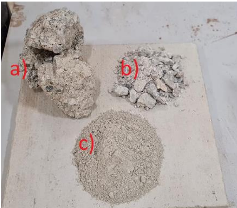
Figure 3.6 Crushing and grinding process of CW. a) Raw form, b) Crushed form, c) Ground form
