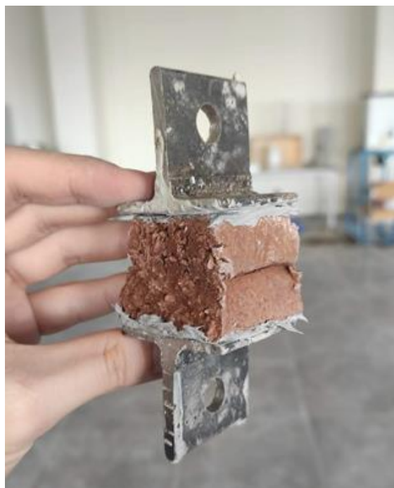
Figure 3.25 Representative image showing glued T-shaped plates on sample
