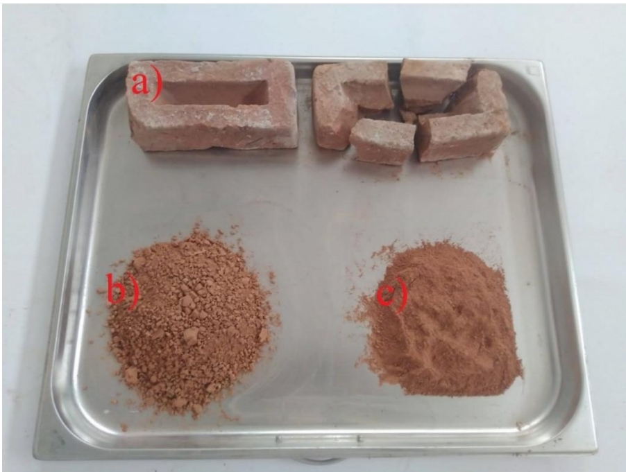
Figure 3.4 Crushing and grinding process of RCB. a) Raw form, b) Crushed form, c) Ground form
