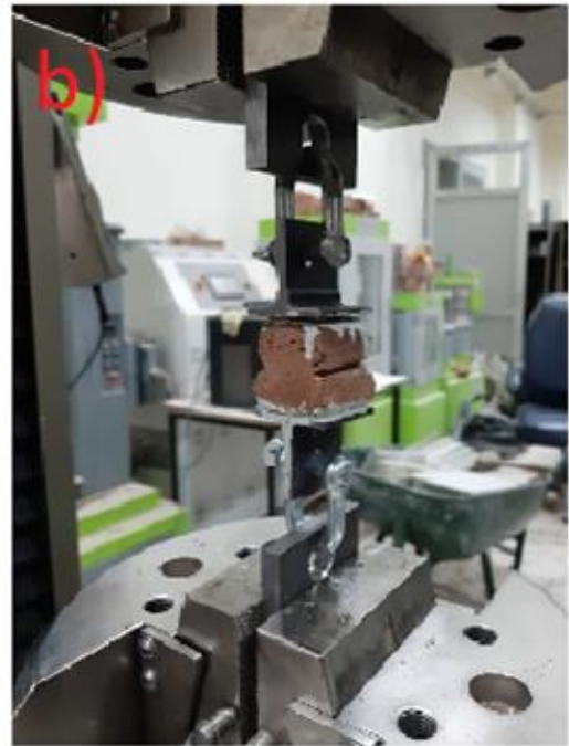
Figure 3.26 Illustration of direct tensile test: a) schematic view, b) test setup
