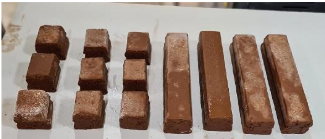
Figure 3.18 Representative images of 3D printed cubic and prismatic specimens curing at ambient conditions
