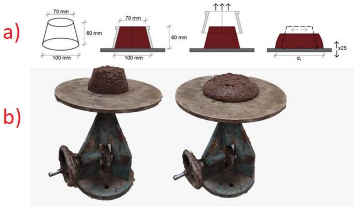
Figure 3.19 a) General schematic view of flow table test, b) illustration of flow table test
