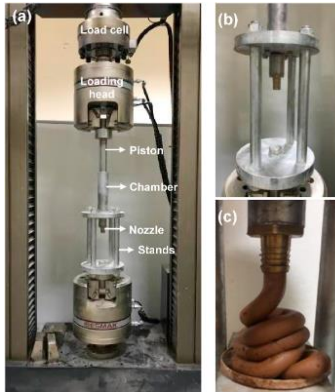
Figure 3.20 a) General view of ram extruder test setup, b) view of nozzle, c) view of extrusion process
