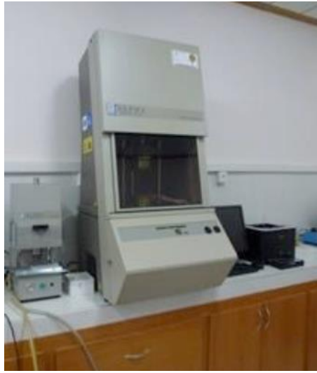
Őekil 3. 5. Alpha Technologies marka MDR cihazı
