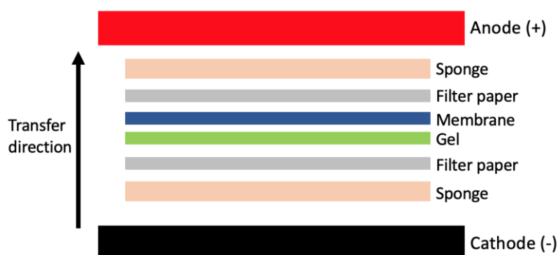
Figure 3.6. Schematic illustration of the western blot wet transfer cassette.
