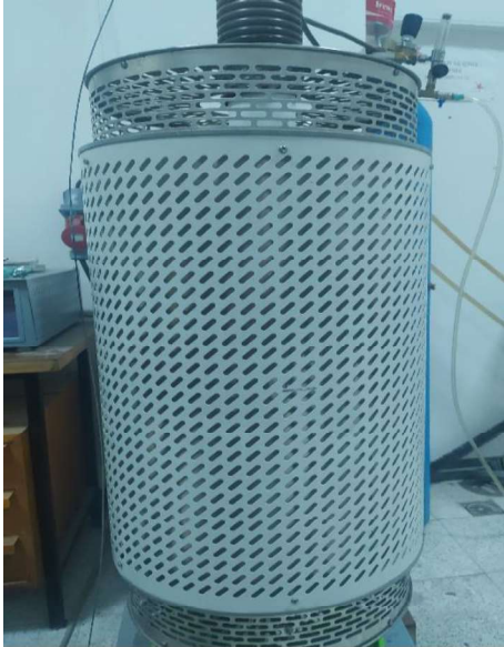
Figure 3.3-2 Cylindrical Furnace that was used for homogenization
