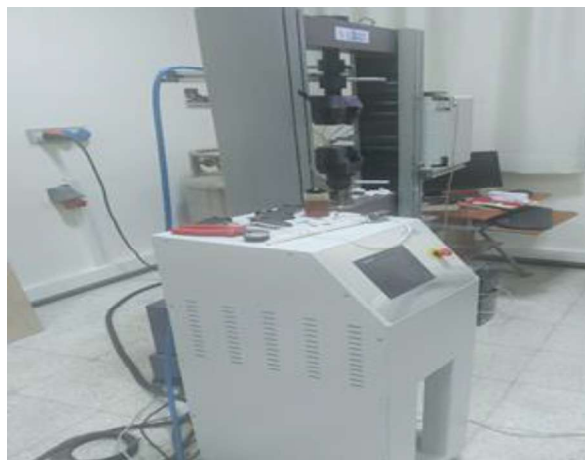
Figure 3.5-1 Utest universal material testing machine equipped with heating/cooling unit that was used for isobaric heating/cooling experiments.
