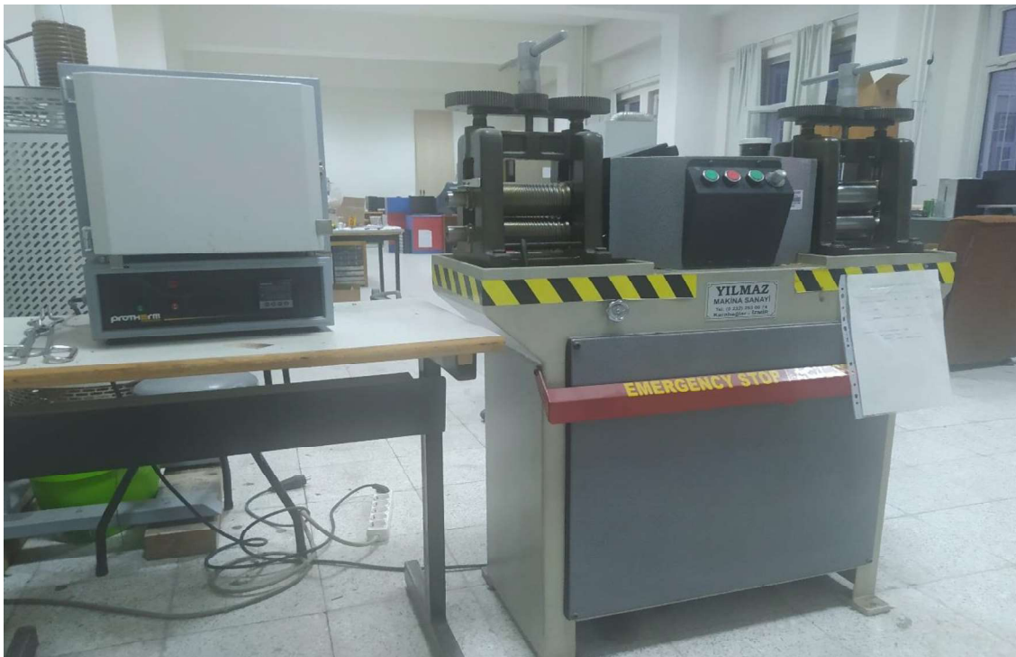
Figure 3.6-1 Cubic Furnace and Rolling Machine
