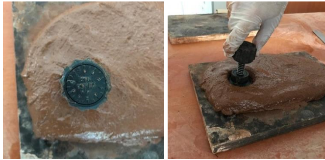
Figure 3.9. Indication of the vane shear device and application of the test
