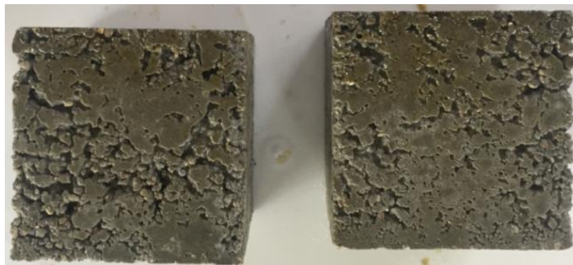
Figure 4. 14. Extremely porous outer surface thought to be related to the settling problem when Bio-2.50% and Bio-3.00% mixtures are removed from the molds.
