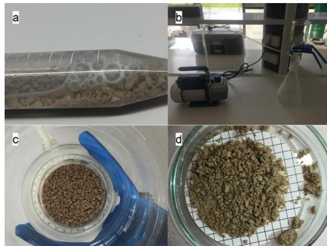
Figure 3. 2. Vacuum filtration test setup to determine water absorption of dry biogranules; (a) dry biogranules soaked in water for 1 h and 24 h; (b) vacuum filtration setup; (c) filtration of non-absorbed water; (d) surface saturated dry biogranules.
