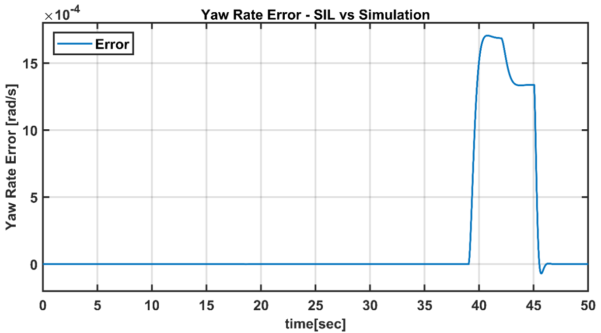
Figure 5-54 SIL test - Yaw rate error
